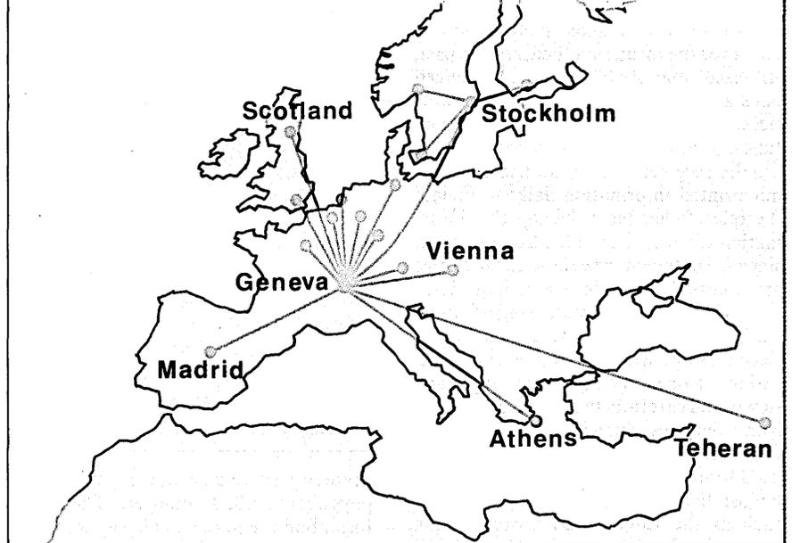
Fig. 2. The network operates in a store and forward mode. In Europe, for example, local sites may perform data base inquiry and update their own files, but must batch all data for files maintained in Geneva. Similarly, Geneva batches data bound for Palo Alto files.
