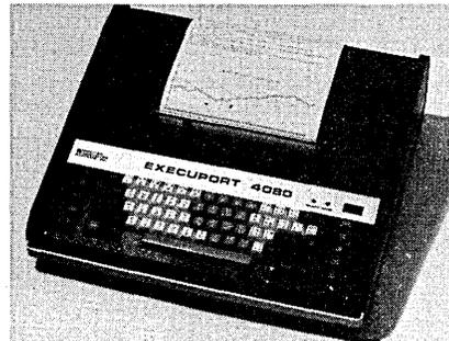
printing of control characters during trouble shooting or program checkout. The print mechanism is capable of limited plotting, with a resolution of 24 points per inch vertically and 10 horizontally. Subscripts, superscripts, underscores, and overscores can be printed; parity errors are identified by printing the bad characters a quarter step above the print line. The 4080 includes an integral acoustic
