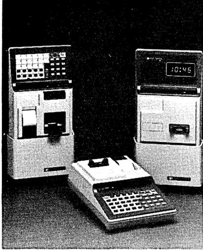
optional. Model 3076A is a wall-mounted version of the 3075A. It can be fitted with a multifunction card reader. One of its applications would be to capture work-in-progress data on a machine shop floor. The 3077A is a wall-mounted time re-
