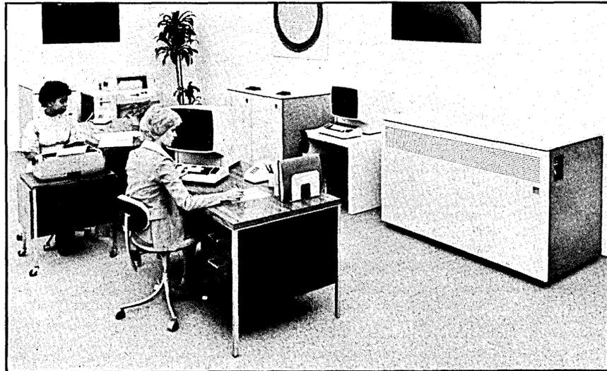
THE 4331 is aimed at the first-time user and can be installed in an office environment. It can be used with currently available IBM I/O and communications devices as well as with the new 3370 disk storage unit shown here.
