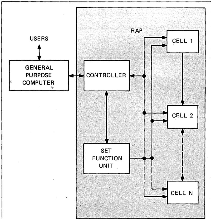
Fig. 3. RAP (Relational Associative Processor) originally was built for a relational data base system, as its name implies, but can be used in other environments as well. Its associative store (cells 1 through N above) is read into a buffer from disk, with mark bits set for those records selected. Records are altered as required while in the buffer, and set functions (summations, etc.) are performed before the data is transmitted to the host.
