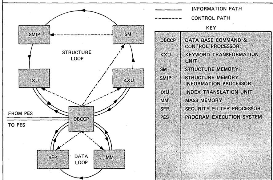
Fig. 4. The DBC (Data Base Computer) was designed to be a slave to a host cpu. It employs microprocessors for each disk track on a cylinder (one for each read head) so an entire memory may be read in parallel, and a pipeline processor architecture so that many processes may be performed on data simultaneously.
