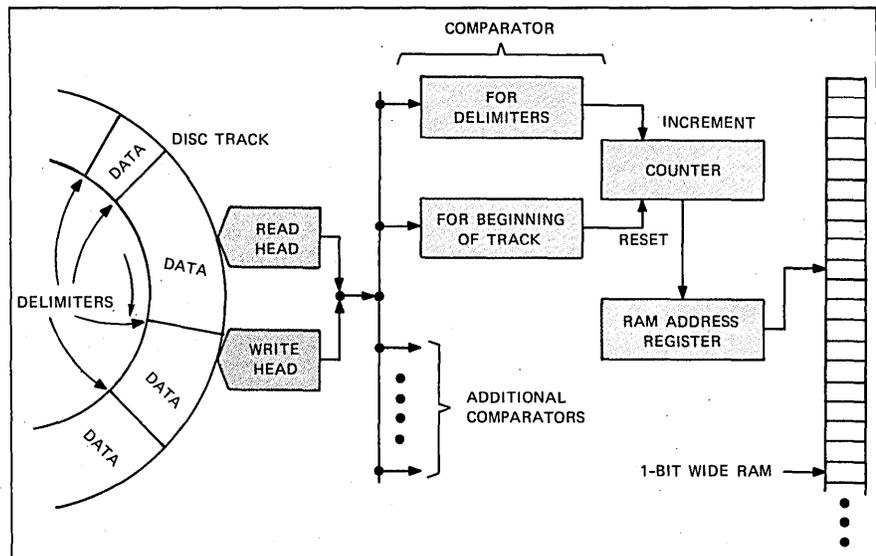
Fig. 2. CASSM (Context Addressable Segment Sequential Memory) was one of the first approaches to a data base processor. Each head on a head per track disk has sufficient logic to test the items recorded on its track, making it possible to search the entire disk in a single rotation, setting the appropriate bit in the RAM for those which meet search criteria.
