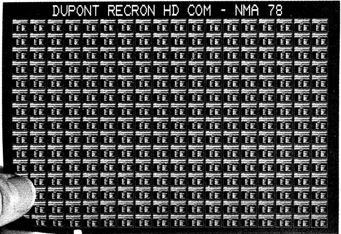
It has brightness, clarity and sharpness that you can actually see. DuPont RECRON High Definition COM silver film has a new emulsion that produces easy-to-duplicate images in reductions of 42x, 48x and higher. That means more information in less space. Wide processing latitude assures you of excellent results under a variety of conditions.
