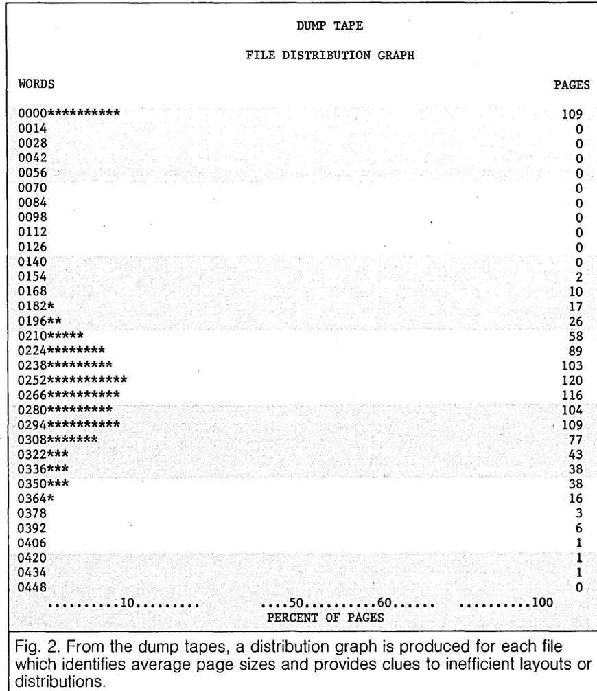
Fig. 2. From the dump tapes, a distribution graph is produced for each file which identifies average page sizes and provides clues to inefficient layouts or distributions.
