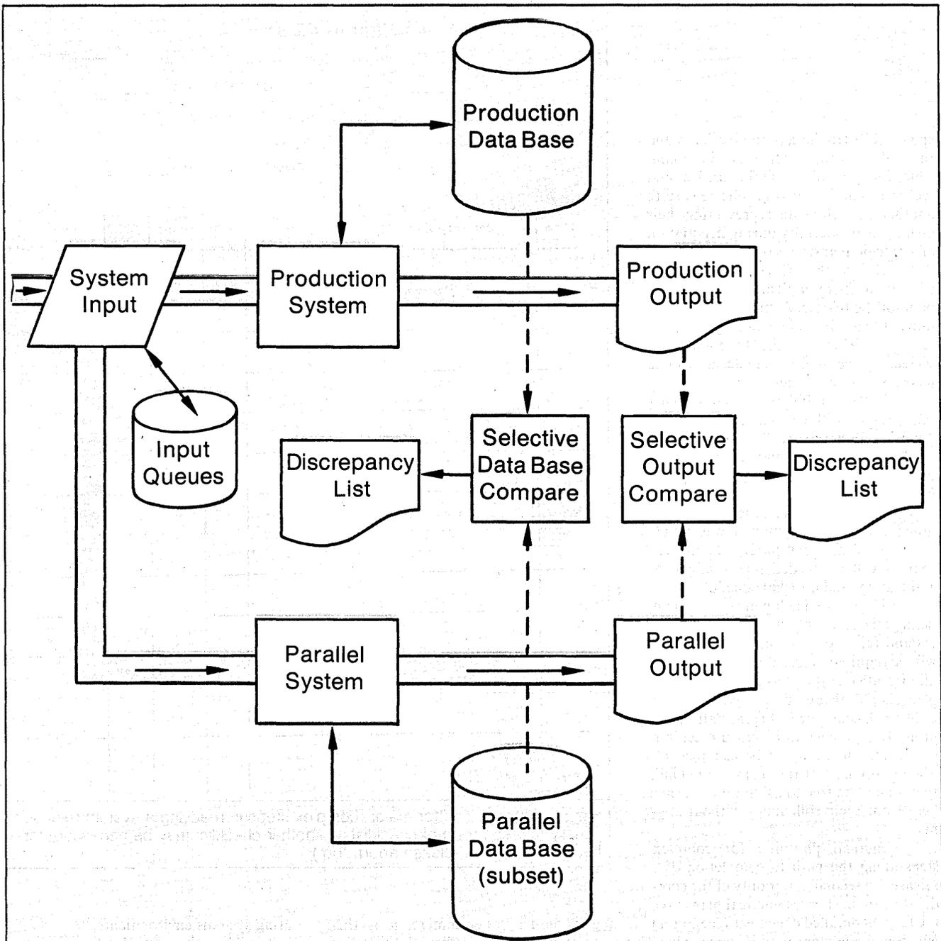
Fig. 2. Running in parallel isn't too difficult for batch systems, but on-line operation complicates the process mightily. The complications are eased by
