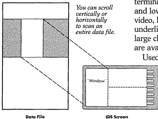
screen can be split into as many as 8 individually controlled and functioning mini displays, each with its own input and output capabilities. Moreover, any one window can be "attached" to a data file and scrolled, both horizontally as well as vertically. Thus, each window
