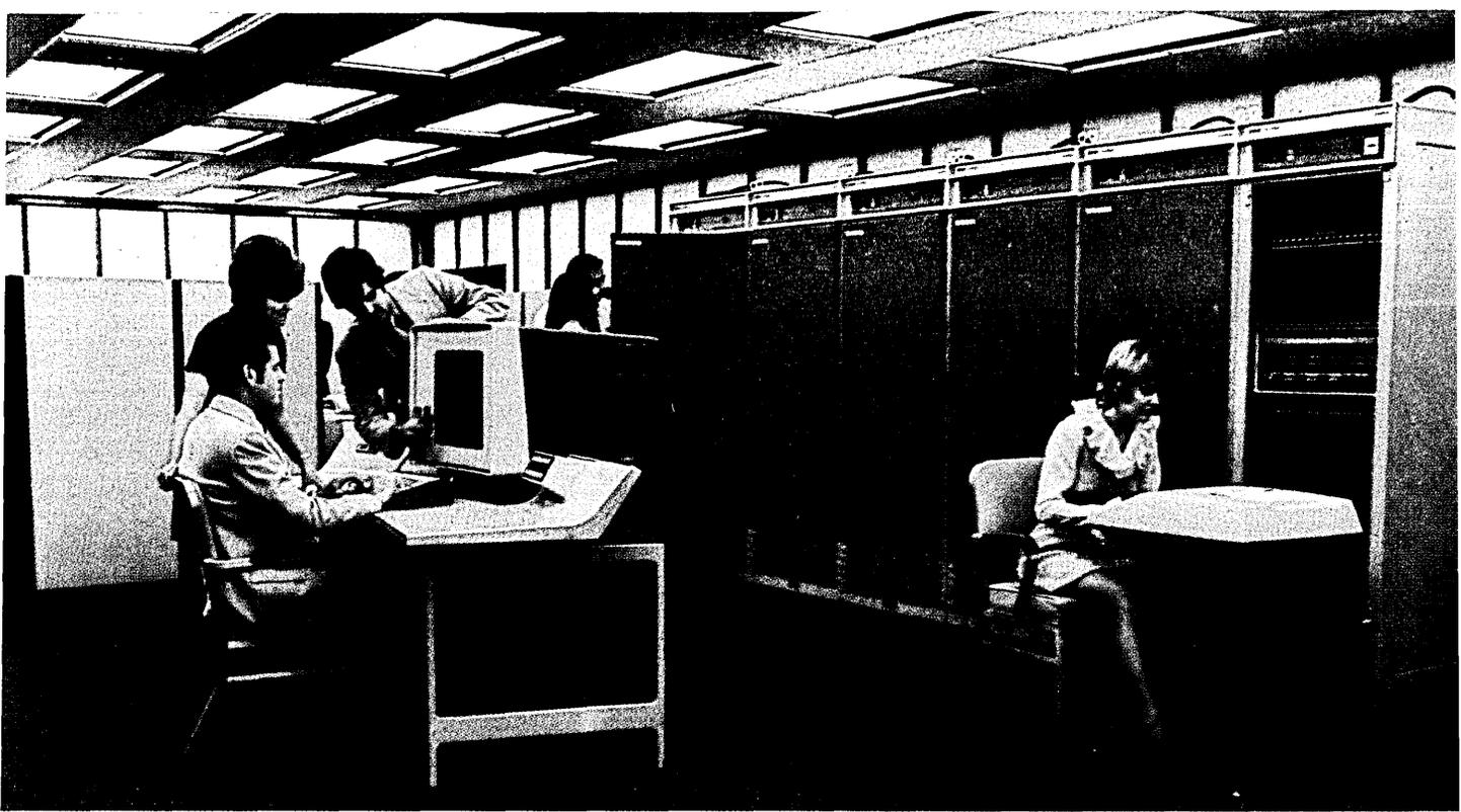
Goodyear Aerospace's STARAN array processor has been marketed for number crunching on high volume scientific applications. Only the one at the Rome Air Development Command has been put to data base work, and that only as a study project.
