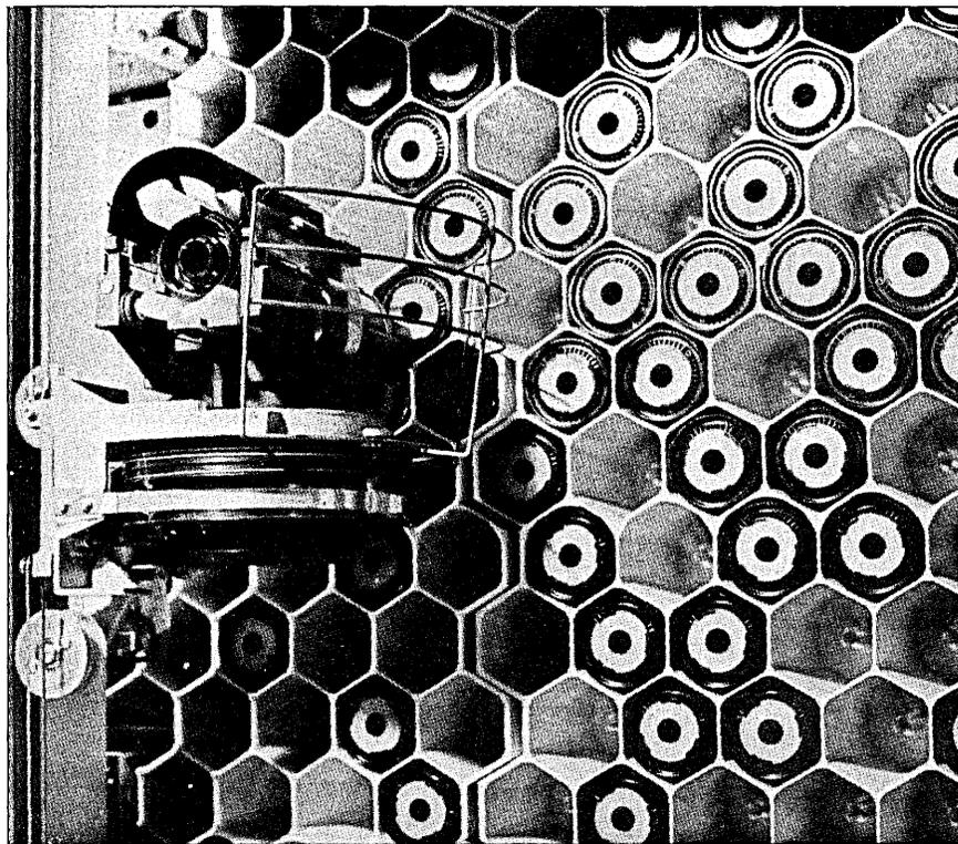
AROUND THE WORLD mass storage systems are going into more shops and at an accelerating rate, although none of the hardware vendors seems to be emphasizing it to any great extent. This is photo of the IBM cartridge storage device that IBM introduced with its 3850 mass storage system in the fall of 1974.
