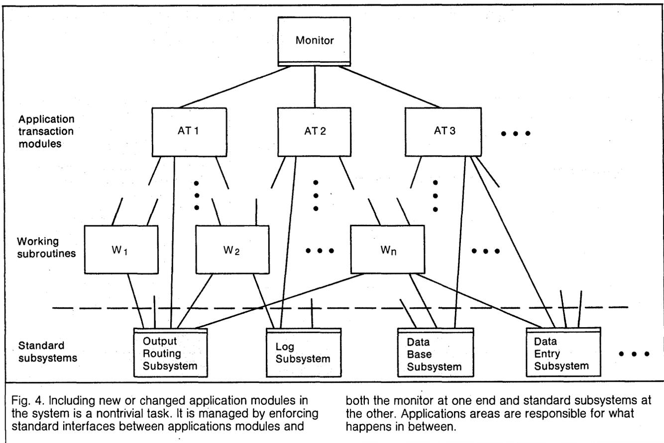
Fig. 4. Including new or changed application modules in the system is a nontrivial task. It is managed by enforcing standard interfaces between applications modules and
