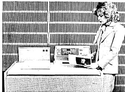
color image—composed of three primary colors—on plain paper. Composite copies are possible using platen (that's the glass window on the copier) or 35mm slide input; the unit can also be used simply as a color copier.
