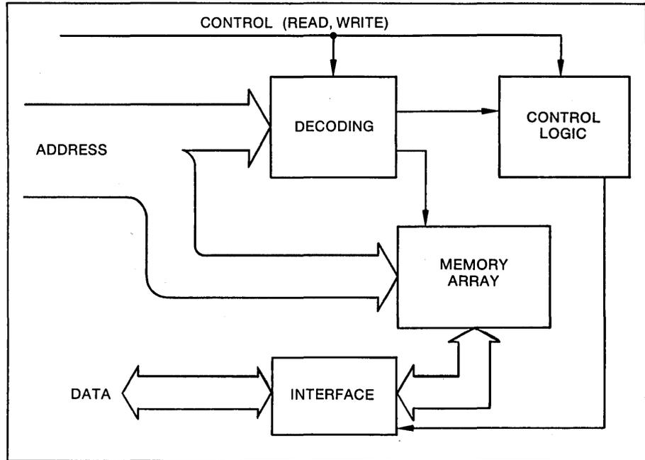
Fig. 3. This illustrates how a typical microcomputer memory system might be organized. Certain bits of the address field are decoded to select elements of the memory array while lower-order bits select words within those elements. Data is read out to or written into those places from the data bus. The control logic might include latches for holding input or output data, refresh circuitry if the memory is dynamic, and so on.
