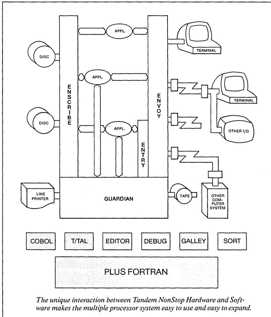
makes it possible to access key-sequenced, relative and entry-sequenced files by primary or up to 255 alternate keys. Provisions have been made to allow exact, approximate or generic positioning into an ENSCRIBE file structure using FORTRAN. Concurrent data base access with other programs and languages is supported with LOCK mechanisms at either the record or file level.
