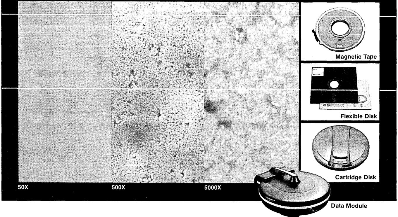
A close look at a section of disk through a scanning electron microscope taken at 50X, 500X and 5000X shows the magnetic oxide coating of the surface. The quality of the surface is of the utmost concern, because of the increasing requirement for higher densities.
