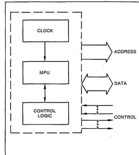
Fig 1. These are the main components of the central processor in a microcomputer. The clock steps the logic from one state to another and synchronizes data transfers. Control logic manages data transfers. In some cases, interrupt logic is also included.
