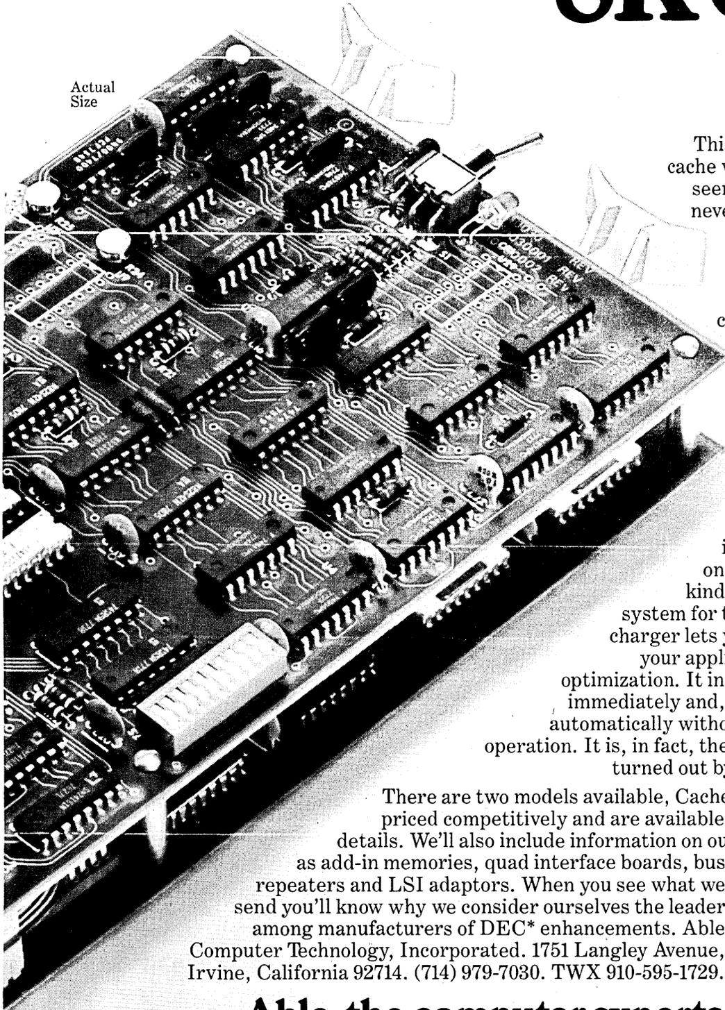
This is the ultimate version, the 8K cache with everything. You have never seen one like it before, and you may never see another. Designed for the 11/34, 11/35 and 11/40, it has byte and address parity, upper/lower limit switches, on-line/off-line manual switch control, activity indicator lights, 8K bytes of memory (4K words) providing a capacity four times that of competitive units and an interconnect board design which consumes no extra space in the computer.
