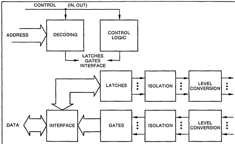
Fig. 4. This illustrates how an I/O subsystem might be organized. Addresses are decoded to select specific ports—which will be sets of logic gates for outputs to the data bus or sets of latches for inputs to the memory.
