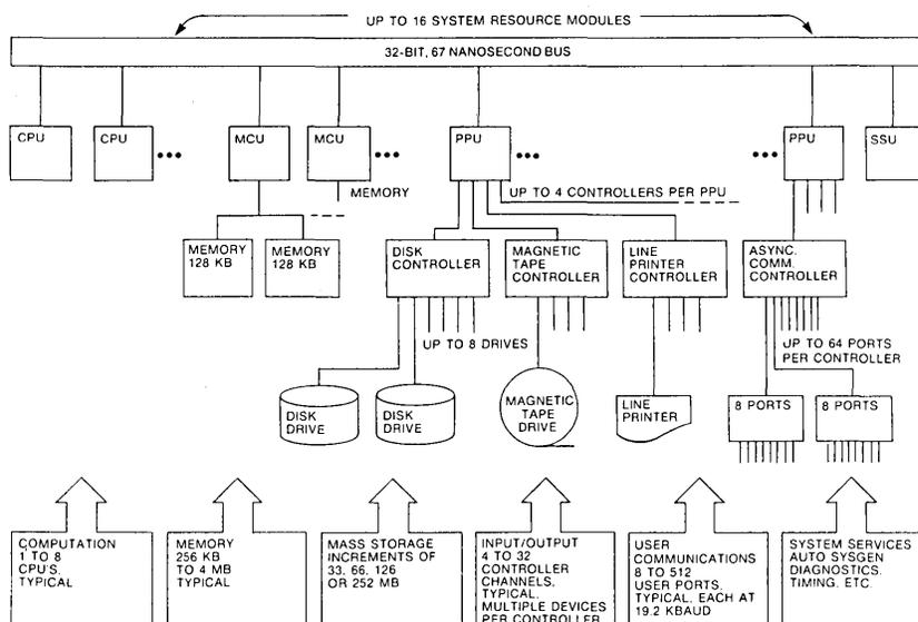
SYSTEM RESOURCE MODULES—FOR COMPUTATION, MEMORY AND I/O—ARE AUTOMATICALLY POOLED FOR EFFICIENT SUPPORT OF INTERACTIVE USERS AND MULTI-STREAM BATCH
