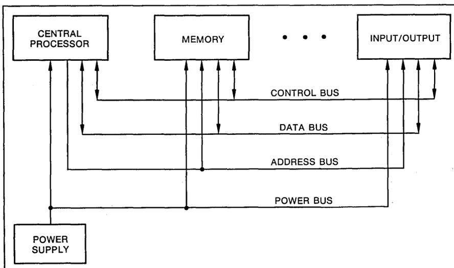
Fig. 5. In modern microcomputers, the cpu, memory, and I/O subsystems are connected by busses for control signals, data, addresses, and power.
