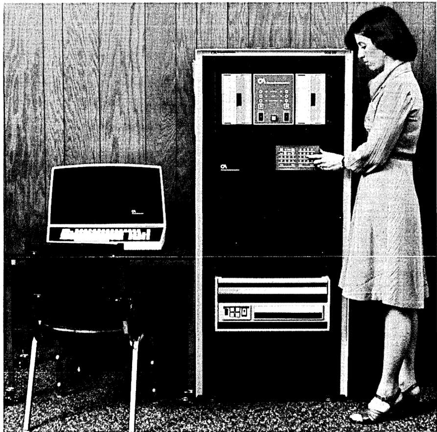
ber are going to 32 bits. Computer Automation's Naked Mini 4 illustrates how broad the range of minisystem packages can be. Available in stripped form (with 4K of memory, power supply, chassis, and console) for \$995, it also can be delivered in configurations like the one above (with hard disc, soft disc, crt, extended memory, etc.). In fact, "typical" systems can run 10 to 15 times as much.
