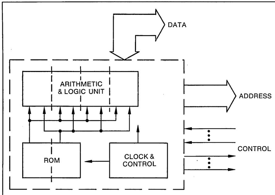
Fig. 2. The microprocessor in a bit-slice microcomputer, as with any other central processor, must have arithmetic and holding registers, the program counter, instruction decoding logic, and sequencing logic. But it also must have a ROM associated with it to store the microprograms used for executing its instructions.
