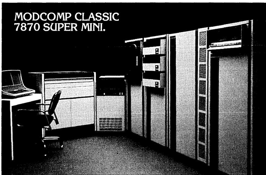
With its large solid state memory (up to 2 million bytes) and an effective memory cycle time as low as 125 nanoseconds, it gives you the speed and capacity you need for demanding scientific, engineering and large process control applications.
