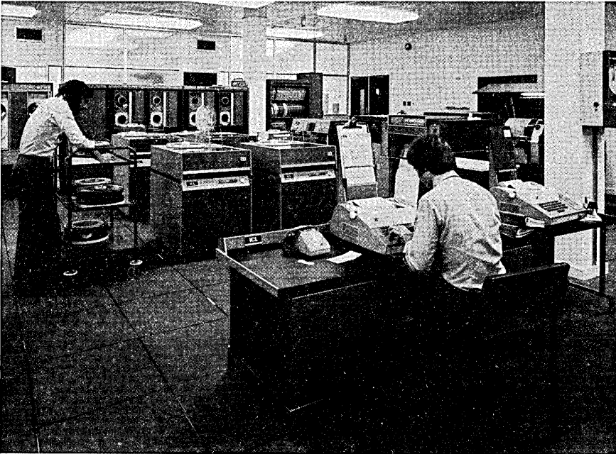
The central site for Vickers' distributed processing operation houses an ICL large scale mainframe (now a model 2960) which links to a continuously changing number of smaller ICL machines (including 2903s and 2904s) at the remote sites. Other Vickers' installations have heavy commitments to non-ICL hardware as well.
