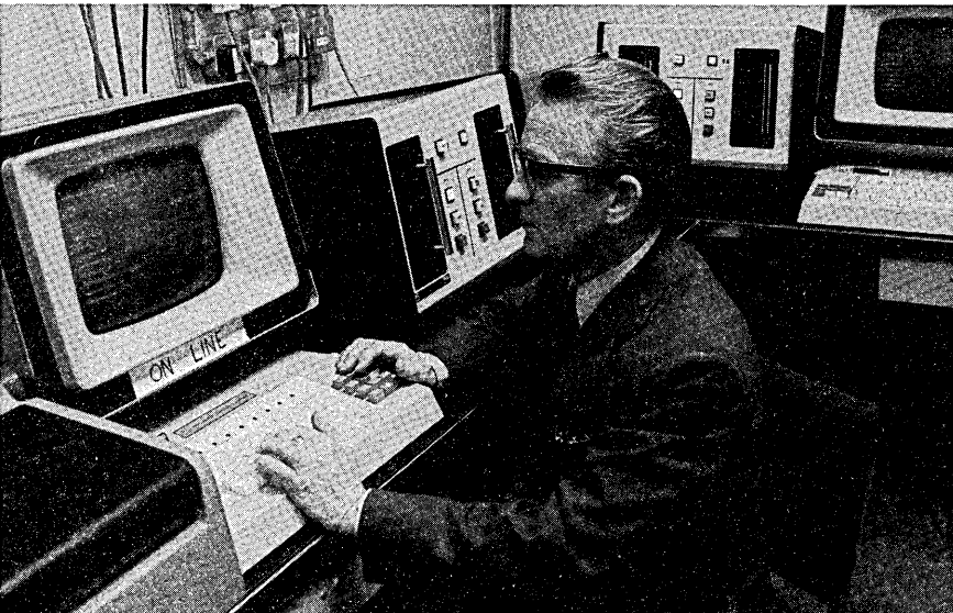
Vickers refers to intelligent terminal sites as Type 3 installations. (For a description of the terminology, see Fig. 1.) The terminal above connects to a small mainframe upstream, and also directly controls a cluster of shop floor terminals downstream.
