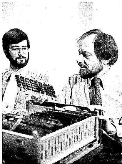
A ZAPP? Sydney Lamb (right) of Semionics with one megabyte associative processor. Box houses microcomputer and 32 cards, each holding 32K bytes of associative memory.
