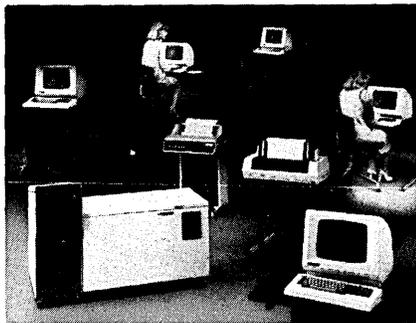
will allow up to nine 445s to be connected over coaxial cable to form a ring network for distributed processing. The package supports shared disc files and the use of remote peripherals.
