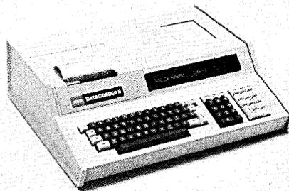
1pm printer, full ASCII keyboard, and an RS232 interface. Peripherals and options include a choice of line printers, 9-track mag tape, an additional cassette drive, external peripheral ports (serial or parallel), and memory expansion to 64KB.
