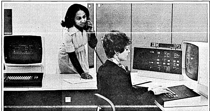
The System 370/3033 is delivered with the cpu, two consoles, a power/coolant distribution unit, and a minimum of 4MB of memory. Said to be 1.6 to 1.8 times as fast, internally, as a 370/168-3, it rents for about 40% less than its predecessor.
