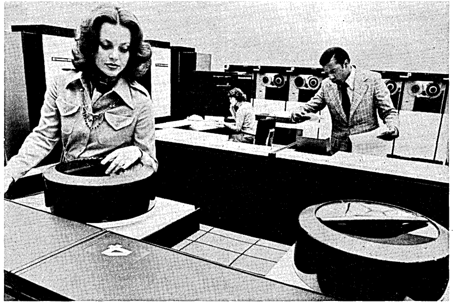
HONEYWELL large-scale Level 66 model, with memory range of 1 million to 4 million bytes, now is offered in Europe and other CII-HB territories along with Level 64 lines. This suggests an overlap with the Level 64 offerings in that territory.
