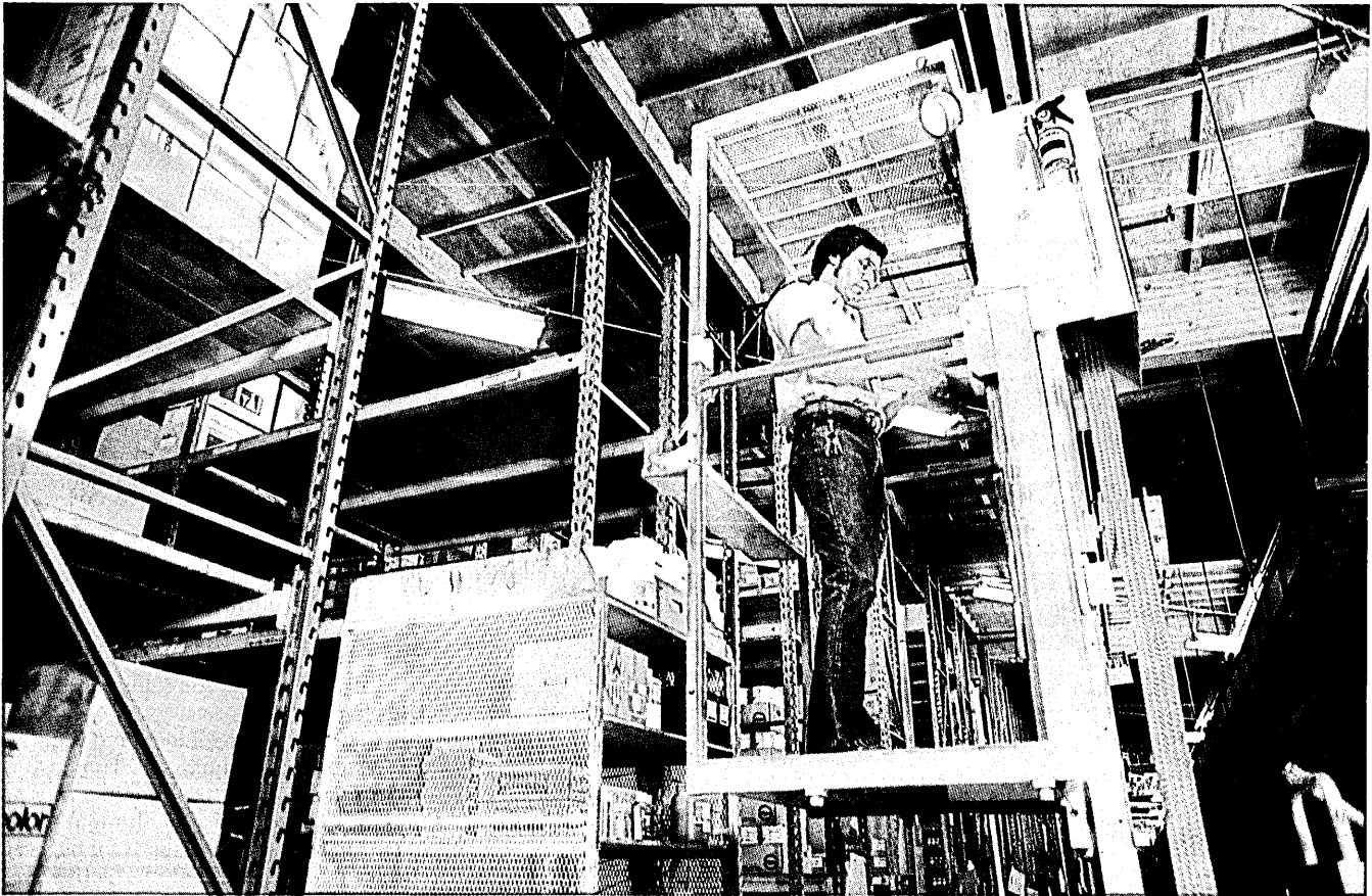
Computer-controlled electric vehicle moves automatically to the selected aisle and bin, for storage and retrieval of goods in a main warehouse of VWR Scientific.
