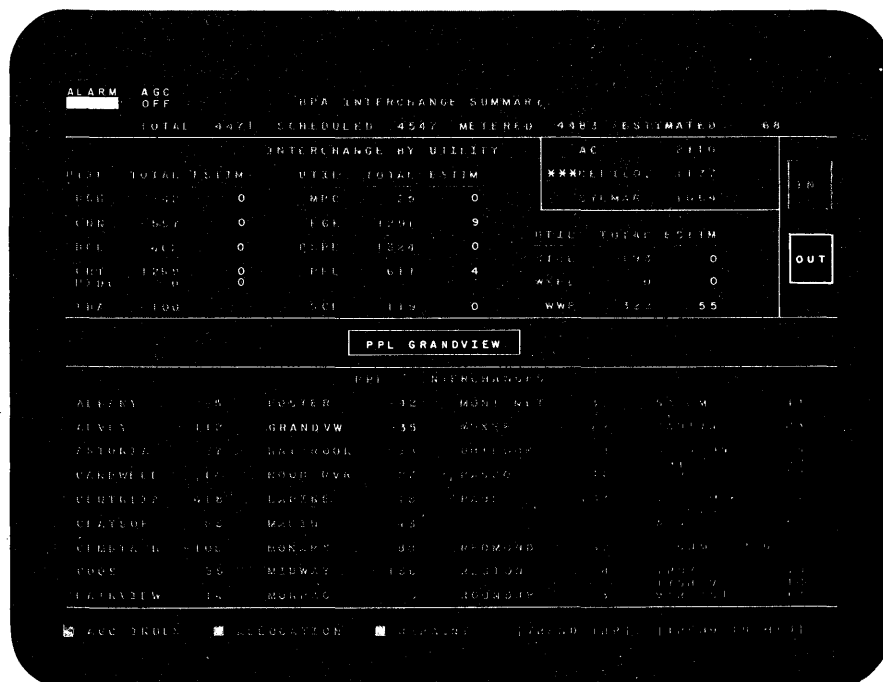
Fig. 2. The interchange summary lists current values for power interchanges with 13 utilities, and the detail of interchange points for one (in this case, Grandview).
