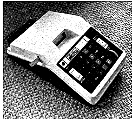
One of the home "terminals" presently used is this one from Theta-Com, the hardware supplier for the Theta-Cable El Segundo experiment.
