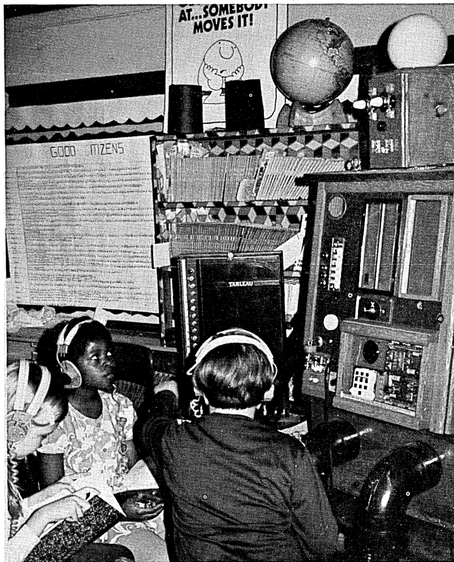
From one to five students can hook into Leachim and each be given personalized attention. The robot interacts through audio input and output, push buttons, and a screen. Its voice, which has purposely been made to sound metallic, has a trace of a Bronx accent.
