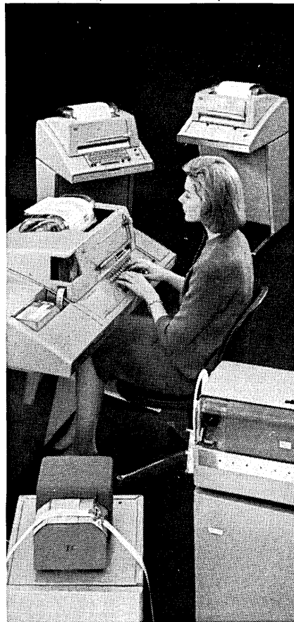
model 35 series: A rugged, heavy-duty line of 100 wpm terminals. Uses ASCII. Units in foreground are self-contained paper tape punch and paper tape reader.
