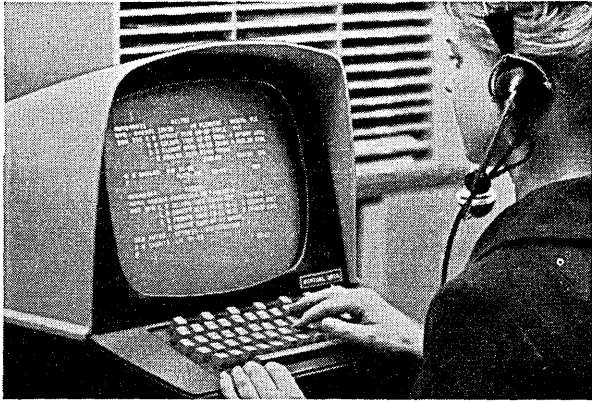
CONTROL DATA 210 Visual Display Unit . . . lets you query the central computer remotely; read out answers instantly on video screen. Up to 63 such units can share a single computer.
