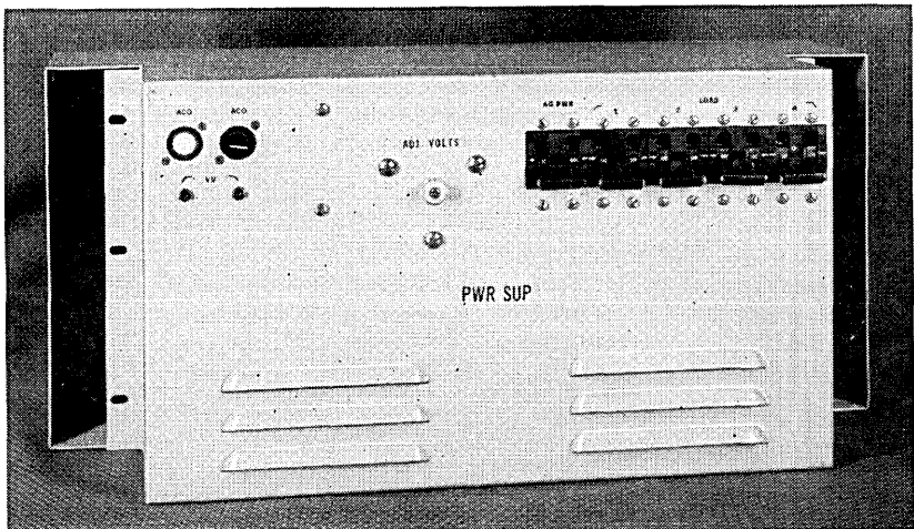
Fig. 19 — Regulator and alarm panel.
