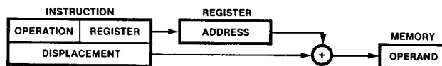
THE OPERAND VALUE IS THE CONTENTS OF THE LOCATION WHOSE ADDRESS IS THE ADDRESS IN THE INSTRUCTION, OFFSET BY THE CONTENTS OF THE REGISTER.
