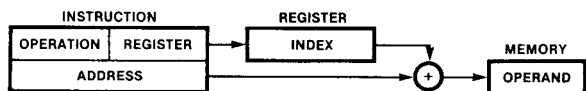
THE OPERAND VALUE IS THE CONTENTS OF THE LOCATION WHOSE ADDRESS IS THE ADDRESS IN THE INSTRUCTION, OFFSET BY THE CONTENTS OF THE REGISTER.
