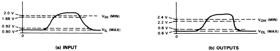
FIGURE 5. VOLTAGE REFERENCE LEVELS
