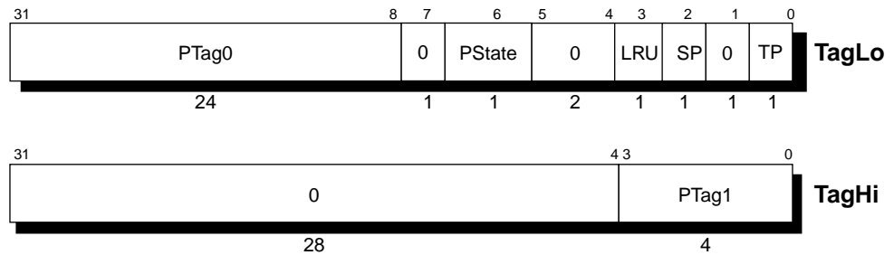
Figure 13-28 TagHi/Lo Register Fields in Primary Instruction Cache When CacheOp is Index Load/Store Tag
