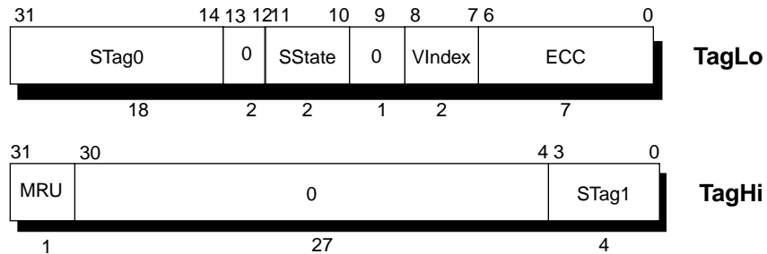
Figure 13-30 TagHi/Lo Register Fields in Secondary Cache When CacheOp is Index Load/Store Tag
