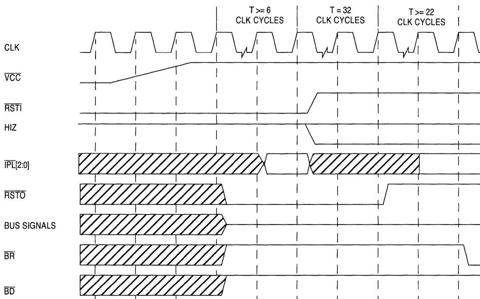
Figure 6-50. Normal Reset Timing
