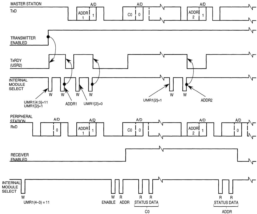
Figure 12-8. Multidrop Mode Timing Diagram
