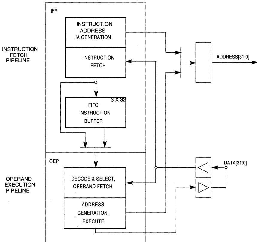
**Figure 3-1. ColdFire Processor Core Pipelines**
