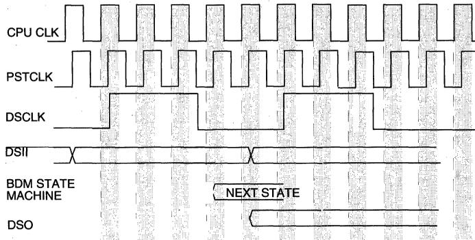
Figure 15-3. DBM Serial Transfer
