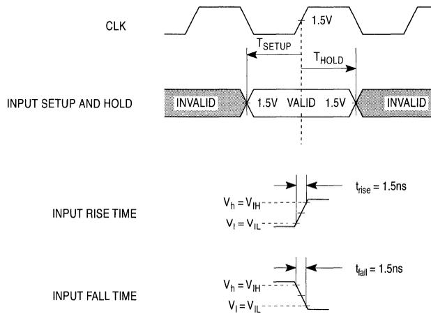
**Figure 17-2. Input Timing Waveform Requirements**
