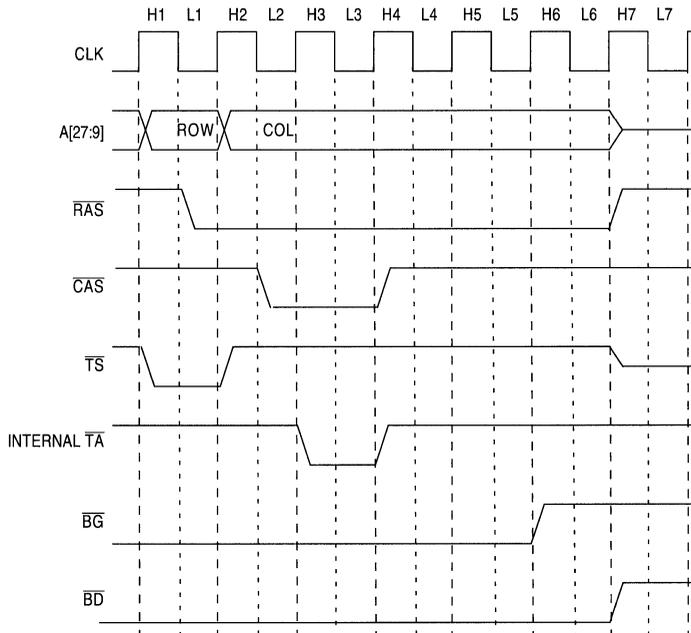
**Figure 11-11. Bus Arbitration in Fast Page Mode**
