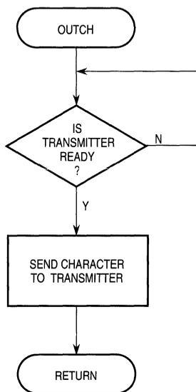
Figure 11-9. UART Software Flowchart (5 of 5)
