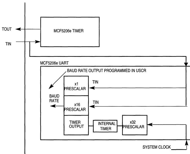
Figure 12-3. Baud-Rate Timer Generator Diagram
