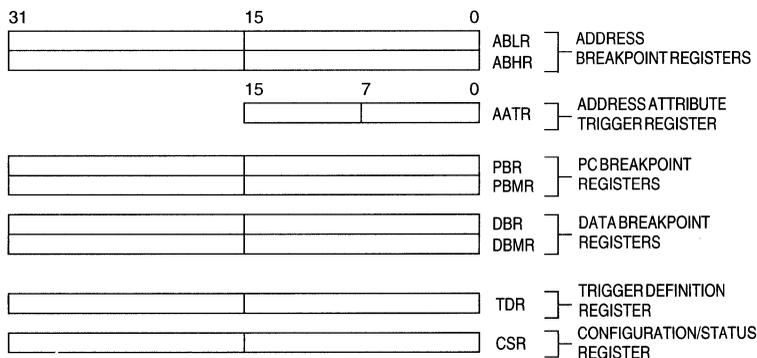
**Figure 15-6. Debug Programming Model**
