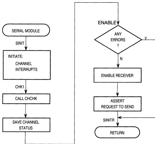
Figure 11-9. UART Software Flowchart (1 of 5)
