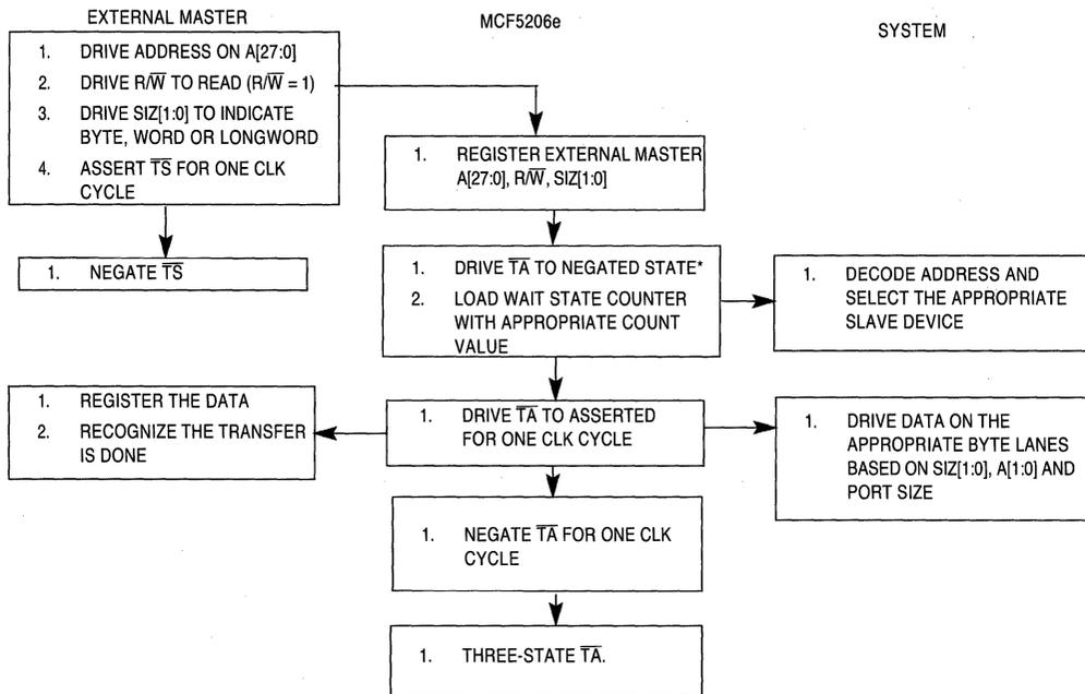
\*TA IS DRIVEN NEGATED IF THE APPROPRIATE WAIT STATE COUNT IS GREATER THAN ZERO. IF THE WAIT STATE COUNT IS ZERO, TA IS DRIVEN AND ASSERTED DURING THE SAME CLK.
