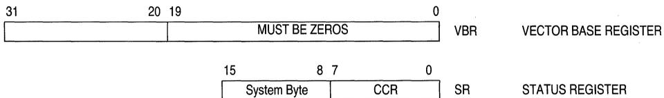
Figure 3-4. Supervisor Programming Model
