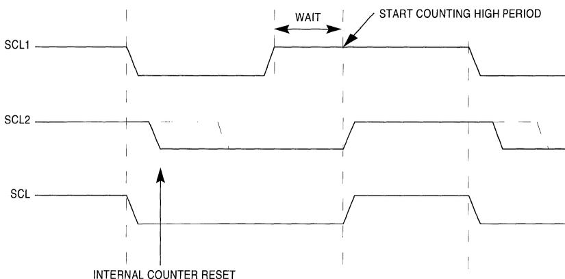
Figure 13-3. Synchronized Clock SCL
