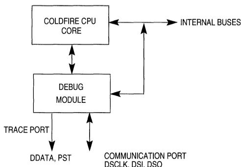
**Figure 15-1. Processor/Debug Module Interface**
