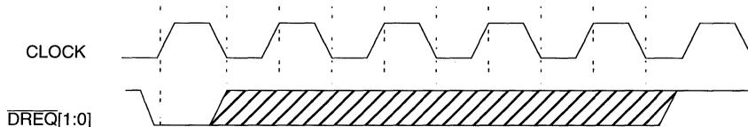
**Figure 7-5. External Request Timing - Cycle Steal Mode, Single-Address Mode**
