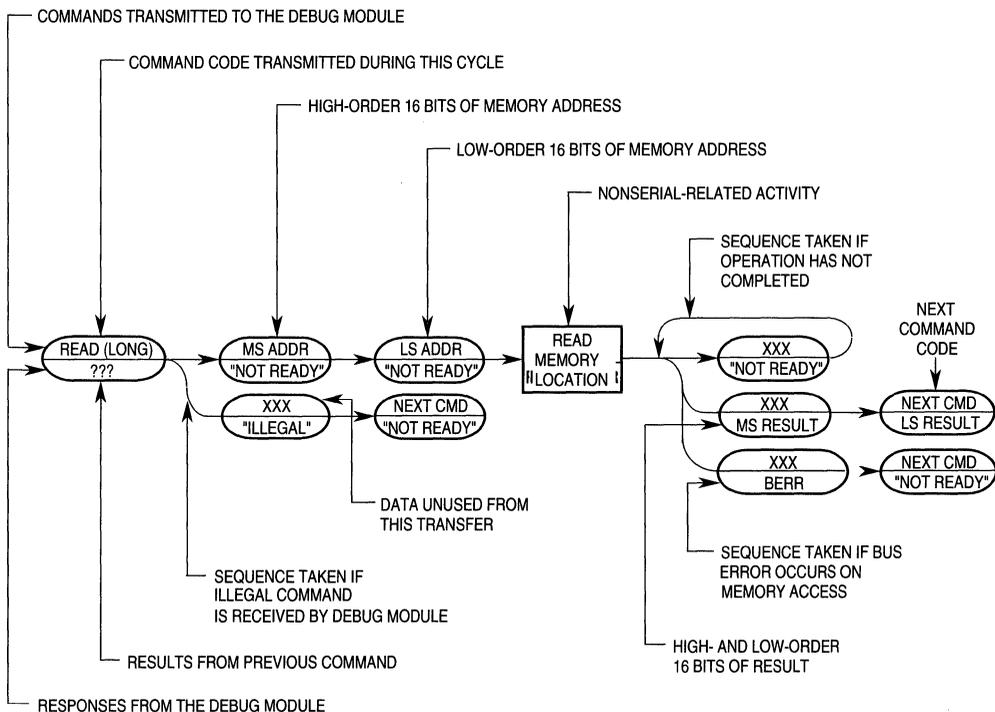
Figure 15-5. Command Sequence Diagram
