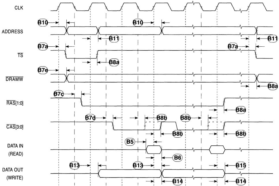
Figure 17-7. DRAM Signal Timing
