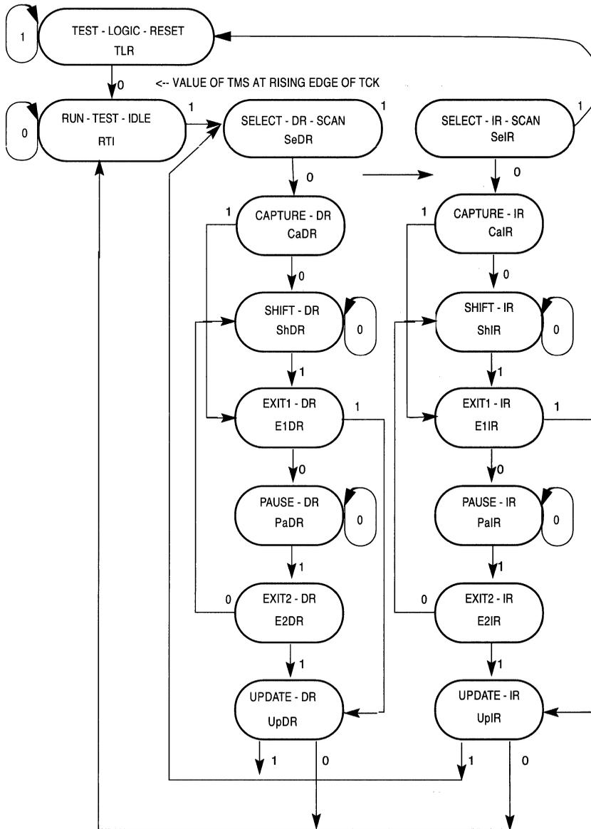
Figure 16-2. JTAG TAP Controller State Machine
