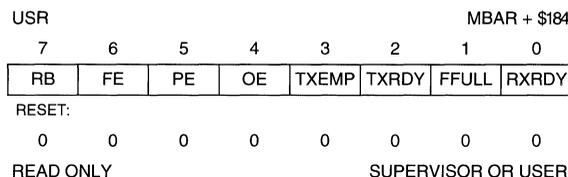
are cleared by the Reset Error Status command in the UCR if the RB bit has not been read. Also, RB, FE, PE and OE can also be cleared by reading the Receive buffer (RE).
