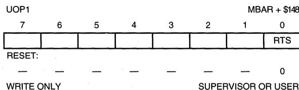
$\overline{\text{RTS}}$  — Output Port Parallel Output
