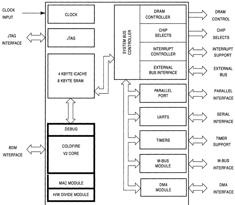
Figure 1-1. MCF5206e Block Diagram
