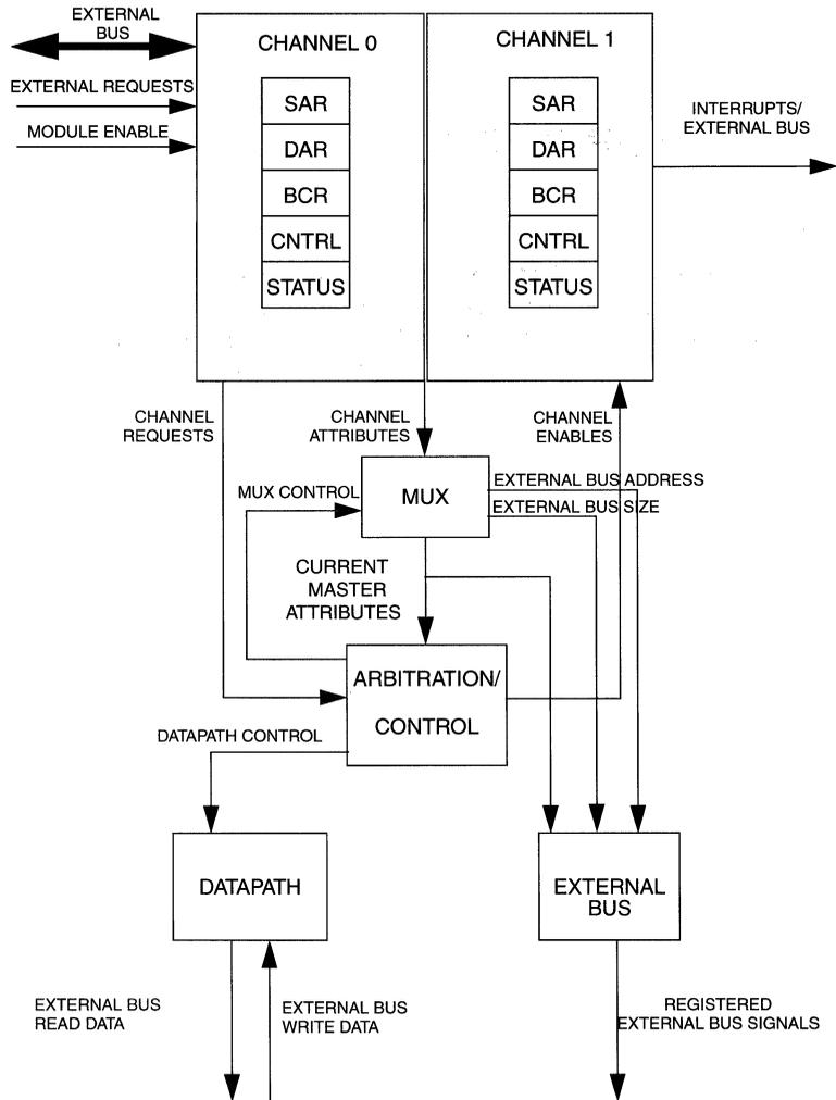
**Figure 7-1. DMA Signal Diagram**
