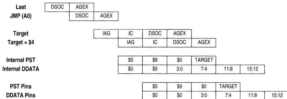
Figure 15-2. Pipeline Timing Example (Debug Output)
