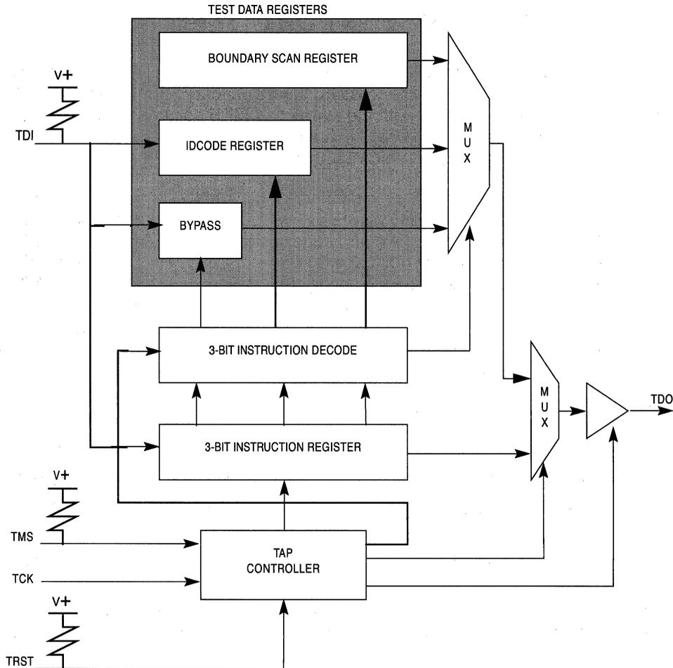
Figure 16-1. JTAG Test Logic Block Diagram
