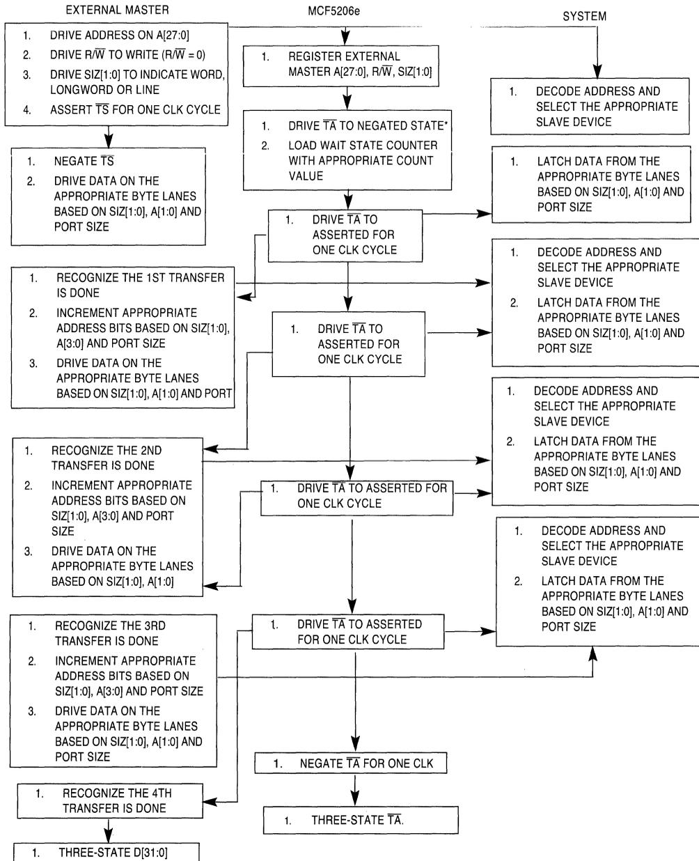
\*TA IS DRIVEN AND NEGATED IF THE APPROPRIATE WAIT STATE COUNT IS GREATER THAN ZERO. IF THE WAIT STATE COUNT IS ZERO, TA IS DRIVEN AND ASSERTED DURING THE SAME CLK.
