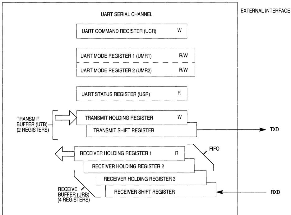
Figure 12-4. Transmitter and Receiver Functional Diagram
