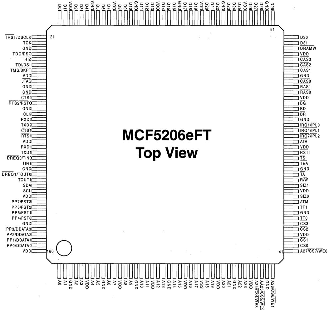
Figure 18-1. MCF5206e Package Diagram & Pinout
