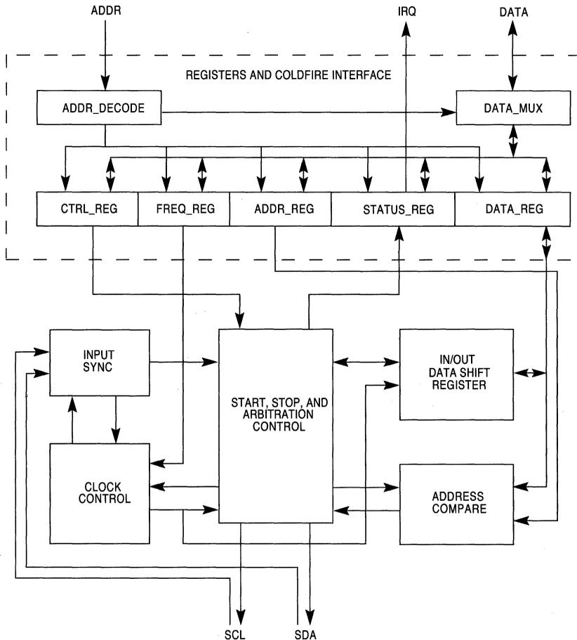
Figure 13-1. M-Bus Module Block Diagram
