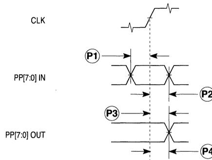
Figure 17-14. General-Purpose I/O Port Timing
