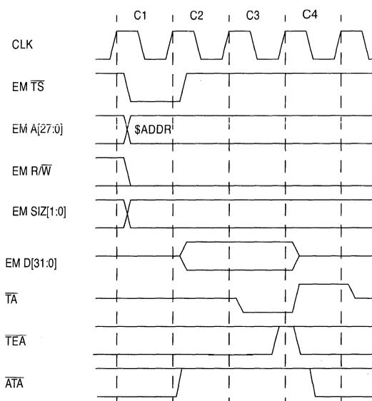
**Figure 6-44. External Master Write Transfer Using MCF5206e Transfer-Acknowledge Timing (No Wait States)**
