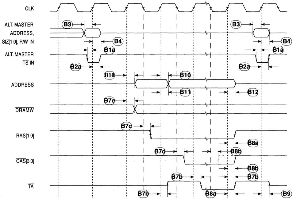
Figure 17-9. DRAM Control By External Master Timing
