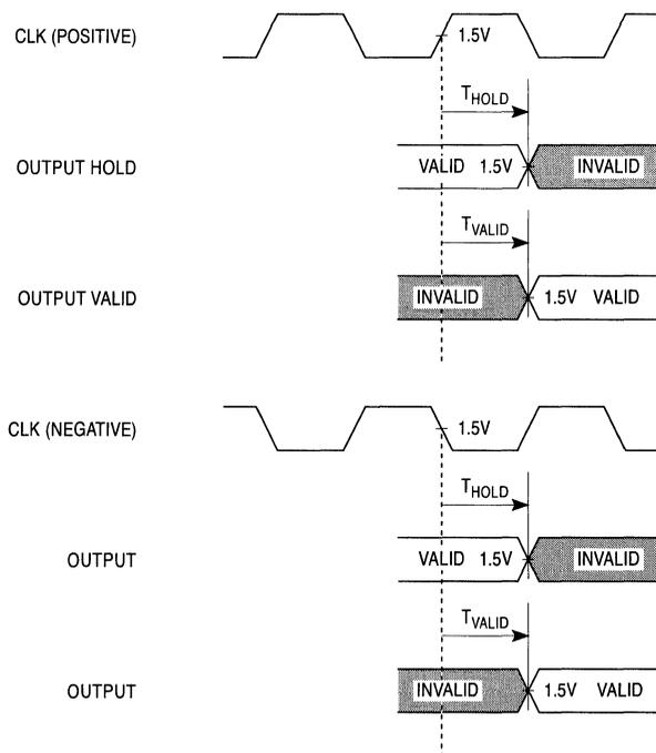
Figure 17-3. Output Timing Waveform
