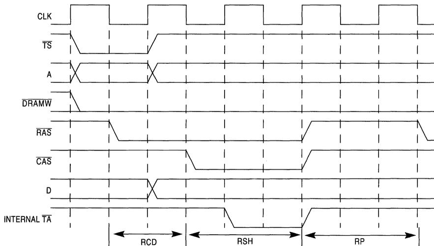
**Figure 11-17. Normal Mode DRAM Transfer Timing**
