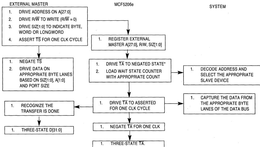
\* $\overline{TA}$  IS DRIVEN AND NEGATED IF THE APPROPRIATE WAIT STATE COUNT IS GREATER THAN ZERO. IF THE WAIT STATE COUNT IS ZERO,  $\overline{TA}$  IS DRIVEN AND ASSERTED DURING THE SAME CLK.
