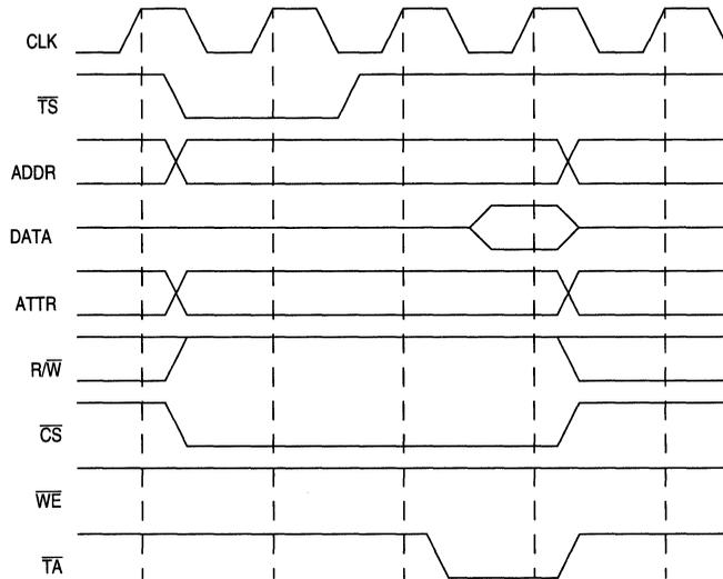
**Figure 9-15. Address Hold Timing with RDAH = 0**
