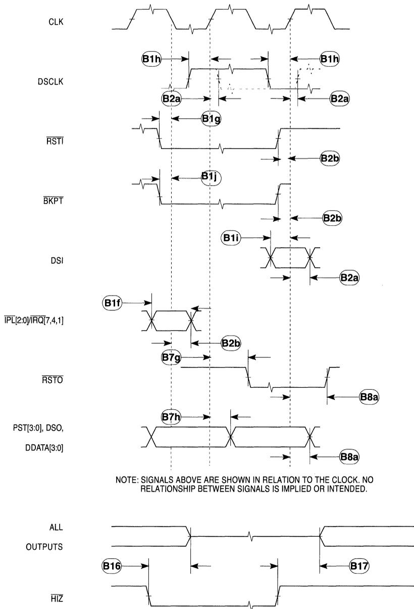
Figure 17-10. Miscellaneous Signal Timing
