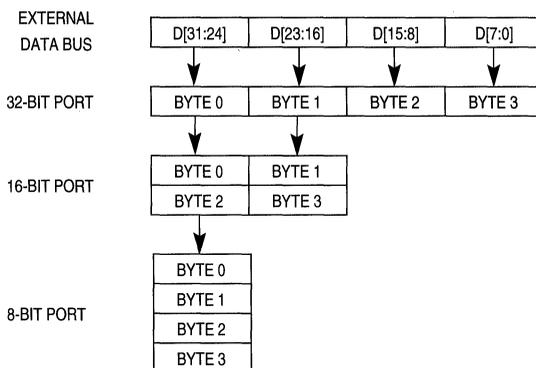
**Figure 9-1. MCF5206e Interface to Various Port Sizes**
