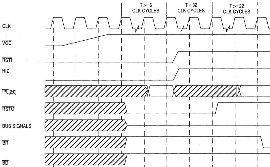
Figure 6-49. Master Reset Timing
