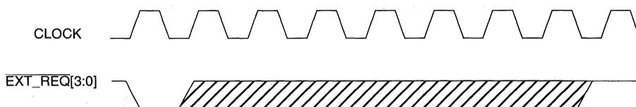
**Figure 7-6. External Request Timing - Cycle Steal Mode, Dual Address Mode**
