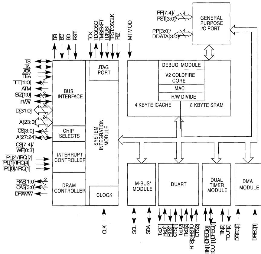
Figure 2-1. MCF5206e Block Diagram
