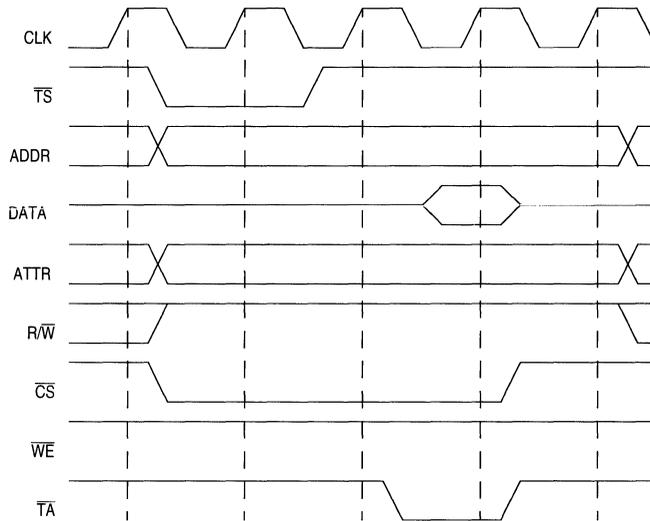
Figure 9-16. Address Hold Timing with RDAH = 1
