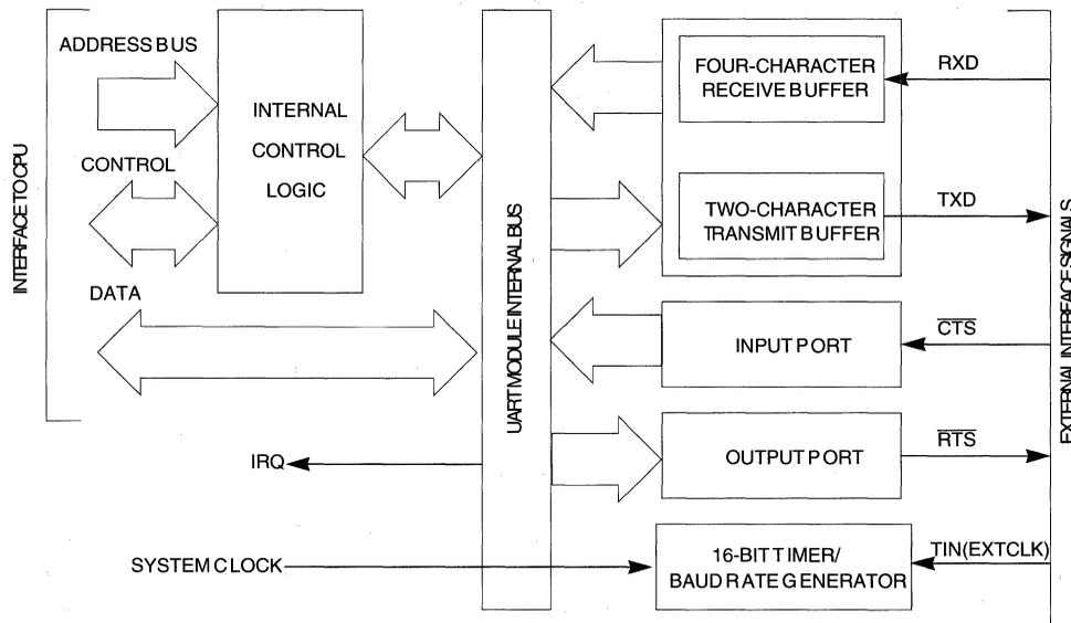
Figure 12-2. External and Internal Interface Signals
