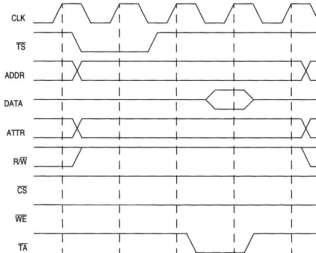
Figure 9-20. Default Memory Address Hold Timing with RDAH = 1
