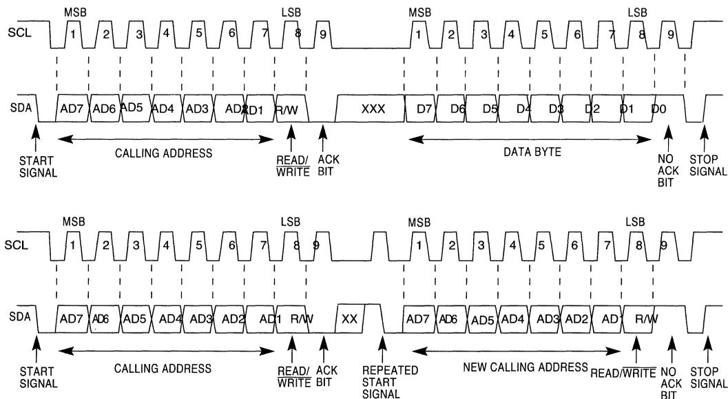
**Figure 13-2. M-Bus Standard Communication Protocol**
