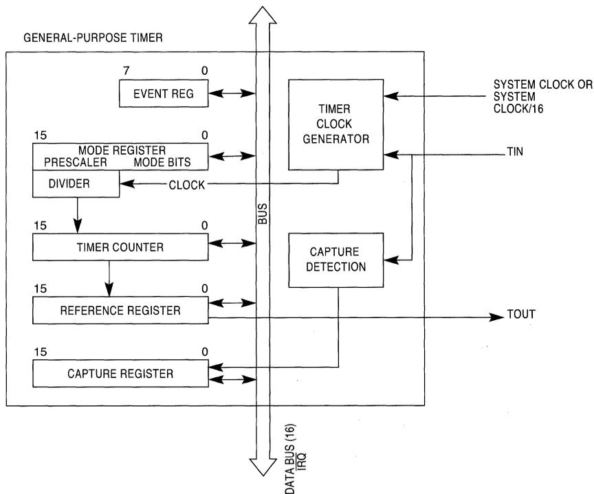
Figure 14-1. Timer Block Diagram Module Operation
