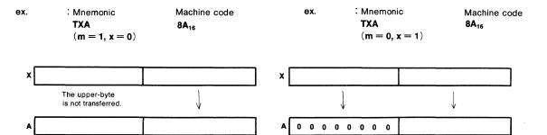
(Note) When the data length differ between the transfer-from and transfer-to locations, data is transferred at the data length for the transfer-to location. If, however, the index register is specified as the transfer-to location and the x flag is set to 1, 0016 is sent as the upper byte value.
