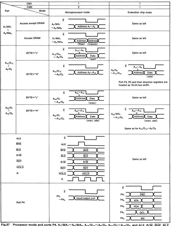
Fig.87 Processor mode and ports P4, A<sub>7</sub>/MA<sub>7</sub>~A<sub>0</sub>/MA<sub>0</sub>, A<sub>15</sub>/D<sub>15</sub>~A<sub>8</sub>/D<sub>8</sub>, A<sub>23</sub>/D<sub>7</sub>~A<sub>16</sub>/D<sub>0</sub>, and ALE, R/W, BHE, BLE, RDY, HOLD, ¢1 functions
