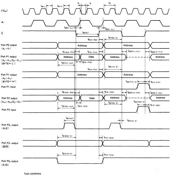
Memory expansion mode and microprocessor mode (When wait bit="1")
