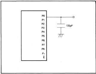
Fig. 4 Testing circuit for ports P0~P8,  $\phi_1$
