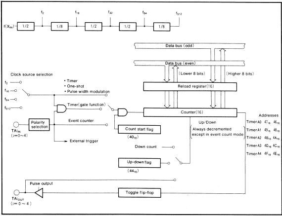
Fig. 11 Block diagram of timer A
