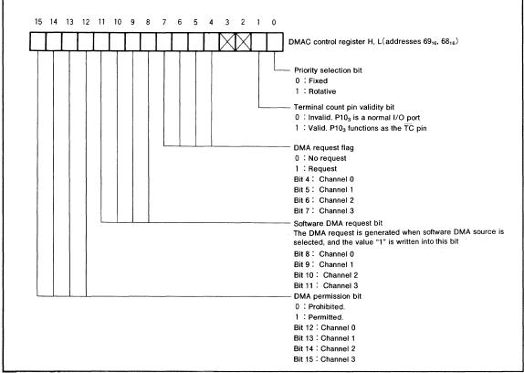
Fig.48 DMAC controll register bit configuration
