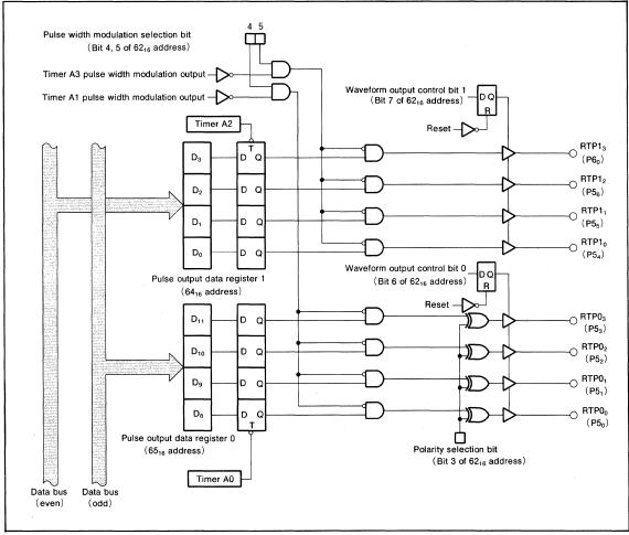
Fig. 33 Block diagram for pulse output port mode
