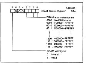
Fig.74 DRAM control register bit configuration
