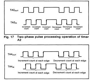
Fig. 18 Two-phase pulse processing operation of timer A4
