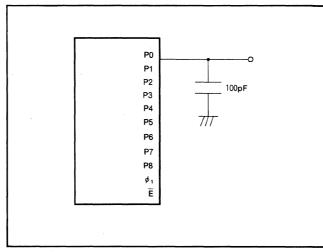
Fig. 3 Testing circuit for ports P0~P8, \$ 1
