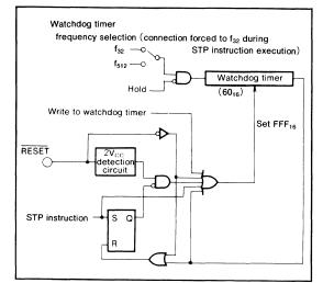
Fig. 52 Watchdog timer block diagram
