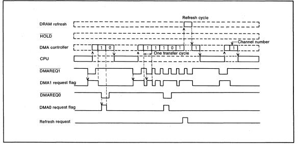
Fig.59 Cycle steal transfer example
