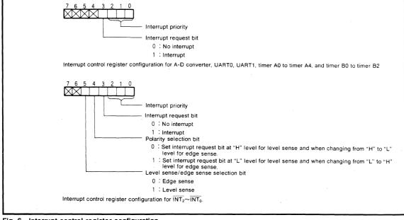
Fig. 6 Interrupt control register configuration
