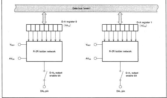
Fig. 50 D-A converter block diagram
