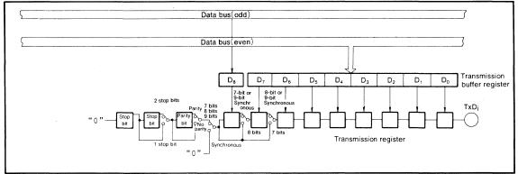
Fig. 41 Transmitter block diagram
