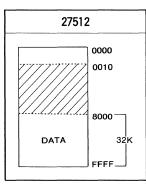
(2) Address  $0_{16}$  to  $10_{16}$  are the area for storing the data on model designation and options. This area must be written with the data shown below. Details for option data are given next in the sec-
