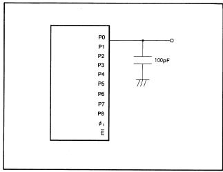
Fig. 5 Testing circuit for ports P0~P8,  $\phi_1$
