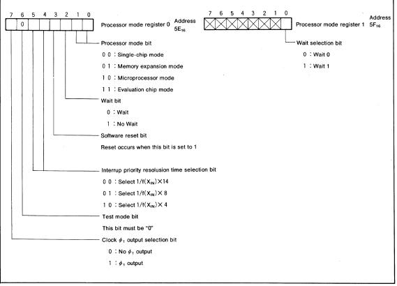
Fig. 58 Processor mode register bit configulation
