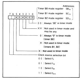
Fig. 28 Timer Bi mode register bit configuration during timer mode
