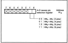
Fig.45 A-D sweep pin selection register configuration
