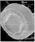
Fig.4 Au-Al plague formation on bonding pad
