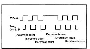
Fig.17 Two-phase pulse processing operation of timers A2 and A3
