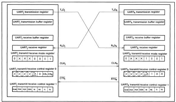
Fig.38 Clock synchronous serial communication
