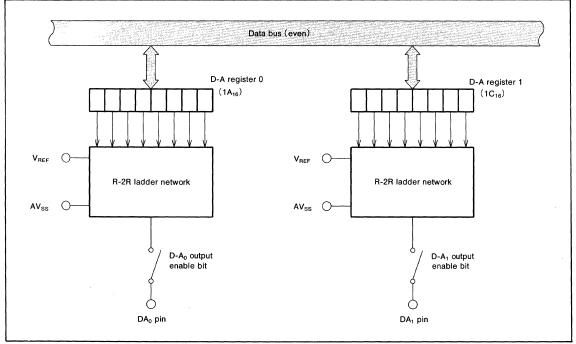
Fig. 50 D-A converter block diagram
