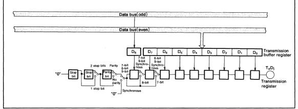
Fig.36 Transmitter block diagram
