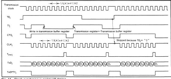
Fig. 44 Clock synchronous serial I/O timing
