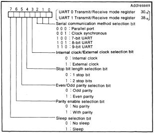
Fig. 39 UART i Transmit/Receive mode register bit configuration
