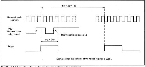
Fig.25 16-bit length pulse width modulator output pulse example
