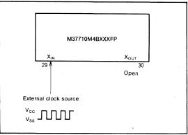
Fig. 64 External clock input circuit
