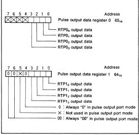
Fig. 36 Pulse output data register bit configuration
