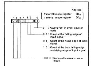
Fig.29 Timer Bj mode register bit configuration during event counter mode
