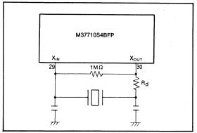
Fig. 63 Circuit using a ceramic resonator
