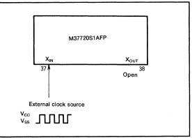
Fig.92 External clock input circuit
