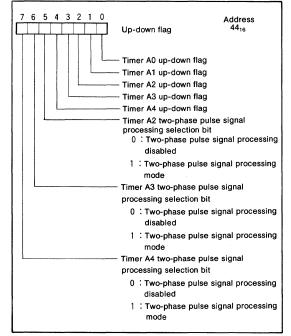
Fig. 16 Up-down flag bit configuration
