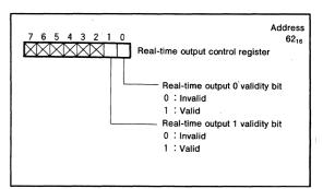
Fig.78 Real-time output control register bit configuration
