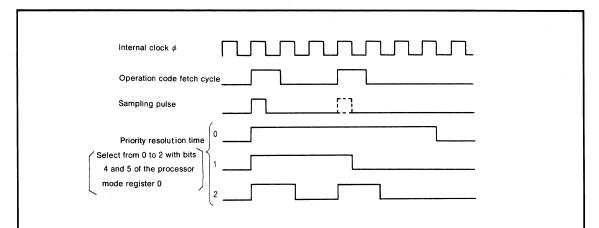
Fig. 9 Interrupt priority resolution time
