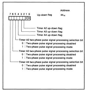
Fig.16 Up-down flag bit configuration
