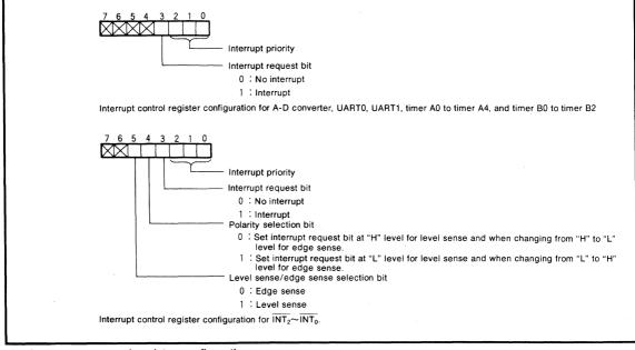
Fig. 6 Interrupt control register configuration
