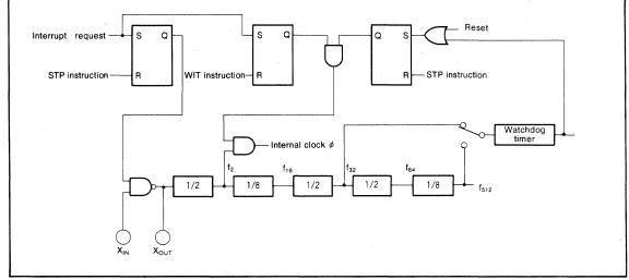
Fig. 62 Block diagram of a clock generator
