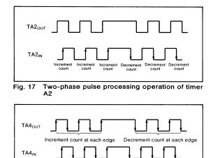
Fig. 18 Two-phase pulse processing operation of timer
