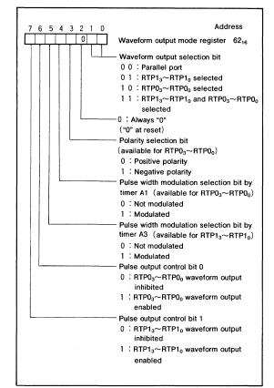
Fig. 34 Waveform output mode register bit configuration
