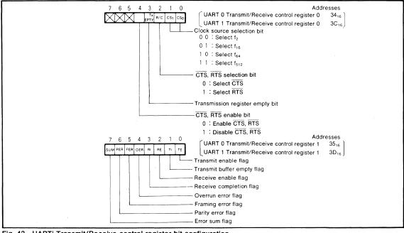
Fig. 42 UARTi Transmit/Receive control register bit configuration
