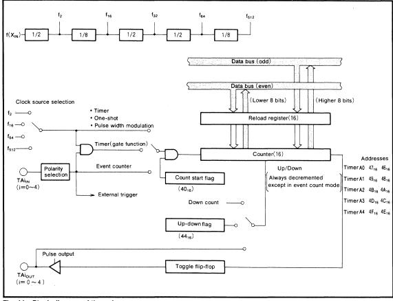
Fig. 11 Block diagram of timer A
