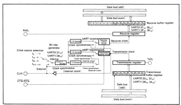
Fig. 38 Serial I/O port block diagram
