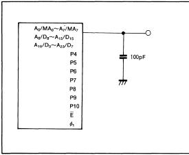
Fig.93 Testing circuit for ports
