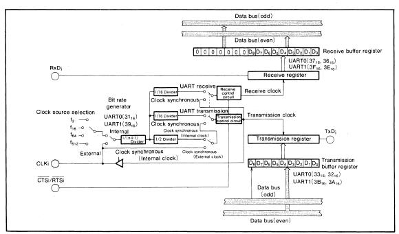
Fig. 38 Serial I/O port block diagram
