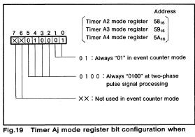
performing two-phase pulse signal processing in event counter mode
