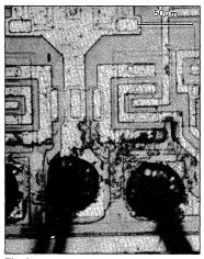
Fig.6 Micrograph of corroded Aluminum metallization
