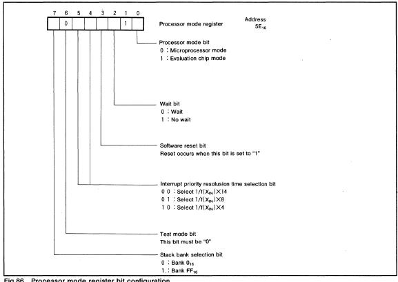
Fig.86 Processor mode register bit configuration
