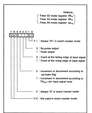
Fig.15 Timer Aj mode register bit configuration in event counter mode
