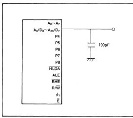
Fig. 65 Testing circuit for each teminal
