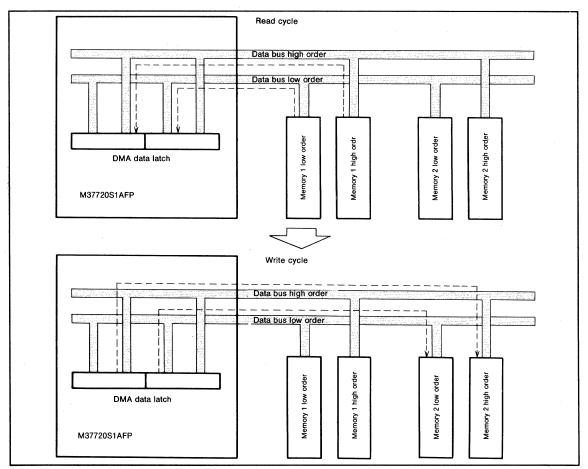
Fig.51 Two bus cycle transfer example
