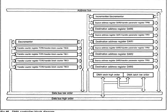
Fig.46 DMA controller block diagram
