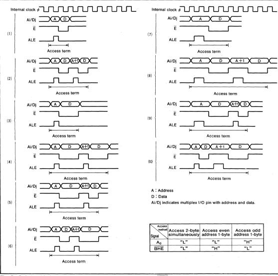
Fig. 5 Relationship between access method and signals  $A_0$  and  $\overline{BHE}$
