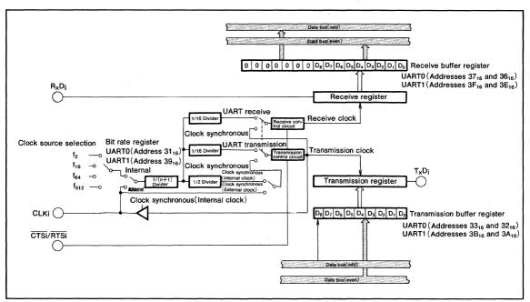
Fig.33 Serial I/O port block diagram
