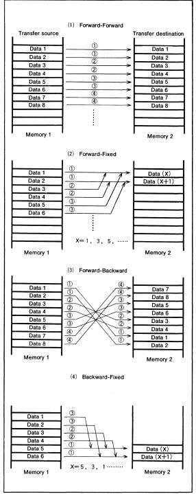
Fig.62 Two bus cycle transfer address change direction examples (when one transfer unit consists of 16 bits)
