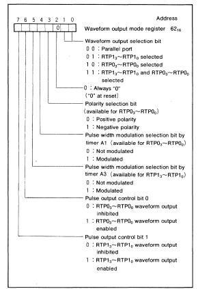
Fig. 34 Waveform output mode register bit configuration
