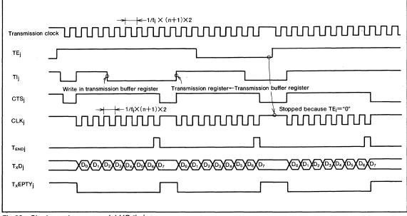
Fig.39 Clock synchronous serial I/O timing
