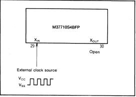
Fig. 64 External clock input circuit
