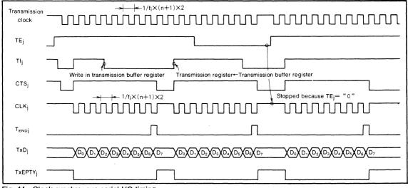
Fig. 44 Clock synchronous serial I/O timing
