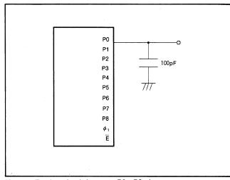
Fig. 65 Testing circuit for ports P0~P8,  $\phi_1$
