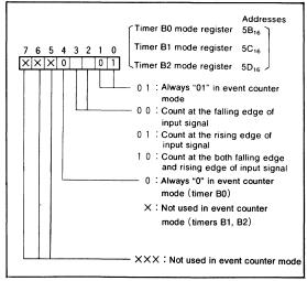
Fig. 29 Timer Bi mode register bit configuration during event counter mode
