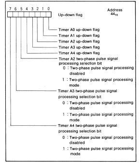
Fig. 16 Up-down flag bit configuration
