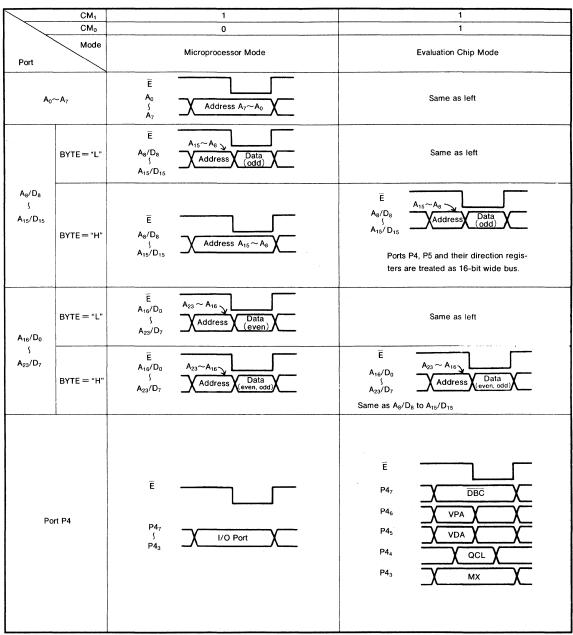
Fig. 59 Processor mode and  $A_0$  to  $A_7$  pins,  $A_8/D_8$  to  $A_{23}/D_7$  pins and port P4 functions
