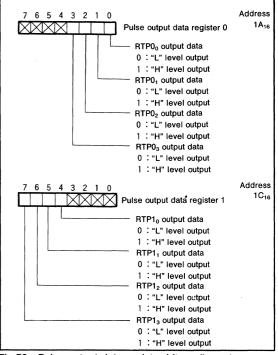
Fig.79 Pulse output data register bit configuration
