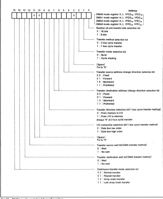
Fig.50 DMAi mode register bit configuration
