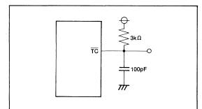
Fig.94 Testing circuit for  $\overline{TC}$  output delay time and  $\overline{TC}$  output pulse width
