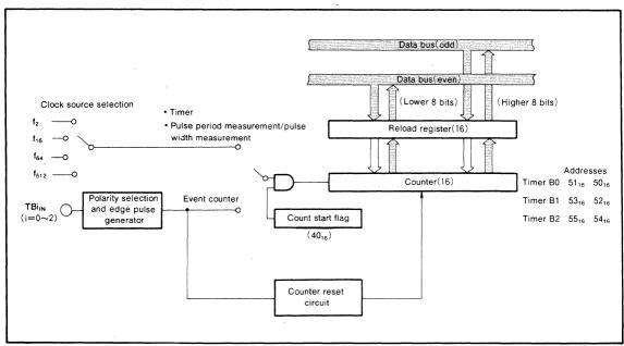
Fig. 27 Timer B block diagram
