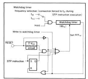
Fig. 52 Watchdog timer block diagram
