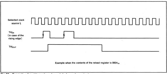
Fig.23 Example when trigger is re-issued during pulse output
