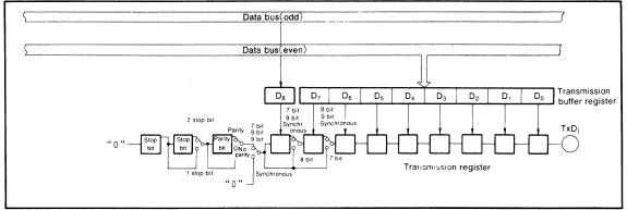
Fig. 41 Transmitter block diagram
