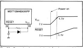
Fig. 55 Example of a reset circuit (perform careful evaluation at the system design level before using)
