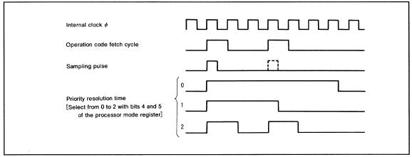
Fig.9 Interrupt priority resolution time
