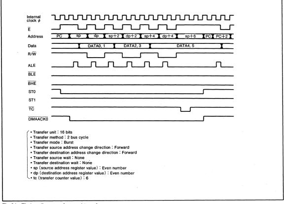
Fig.64 Timing diagram of normal transfer
