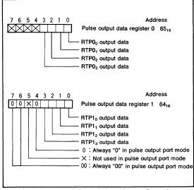
Fig. 36 Pulse output data register bit configuration
