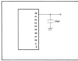
Fig. 3 Testing circuit for ports P0~P8,  $\phi_1$
