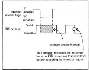
Fig. 10 INTi interrupt during level sense mode
