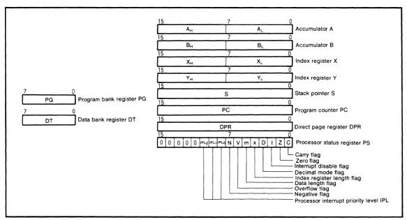
Fig. 3 Register structure
