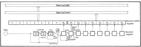
Fig. 40 Receiver block diagram
