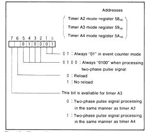
Fig. 19 Timer Aj mode register bit configuration when performing two-phase pulse signal processing in event counter mode
