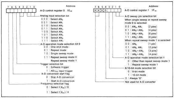
Fig. 49 A-D control register bit configuration
