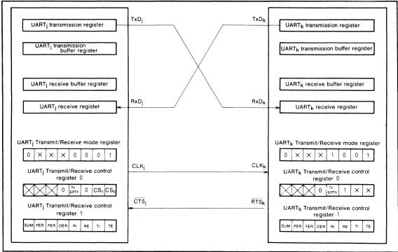
Fig. 43 Clock synchronous serial communication
