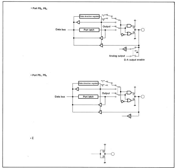
Fig. 57 Block diagram for ports P8 to P4 and E pin output (2)
