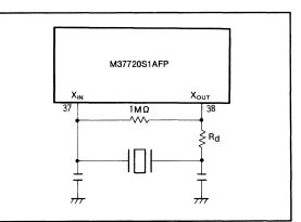
Fig.91 Circuit using a ceramic resonator
