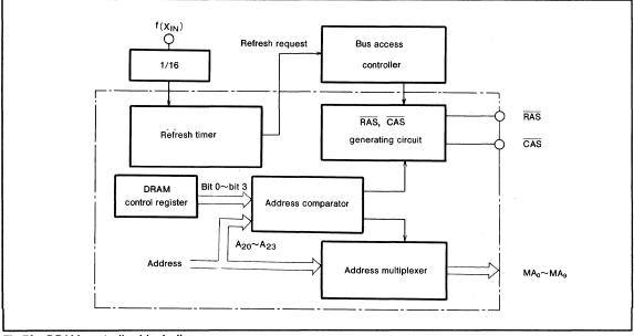
Fig.73 DRAM controller block diagram
