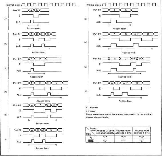
Fig. 5 Relationship between access method and signals  $A_0$  and  $\overline{BHE}$
