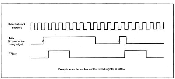
Fig.22 Pulse output example when external rising edge is selected
