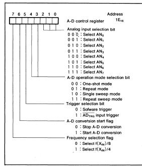
Fig.44 A-D control register bit configuration
