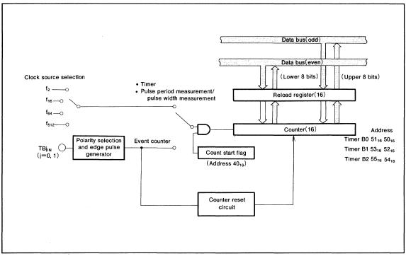
Fig.27 Timer B block diagram
