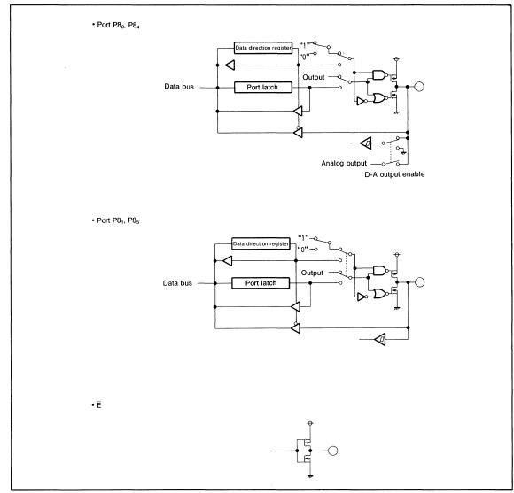
Fig. 57 Block diagram for ports P8 to P0 in single-chip mode and  $\overline{E}$  pin output (2)
