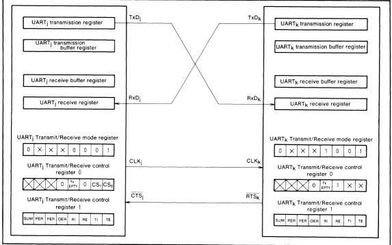
Fig. 43 Clock synchronous serial communication
