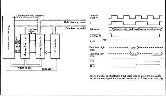
Fig.54 1 bus cycle transfer example(memoly to I/O)(2)
