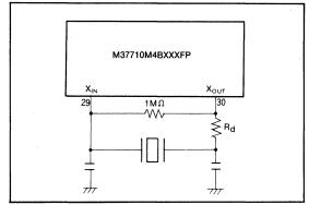
Fig. 63 Circuit using a ceramic resonator
