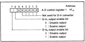
Fig. 51 A-D control register 1 bit configuration
