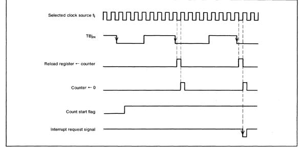
Fig.31 Pulse period measurement mode operation
