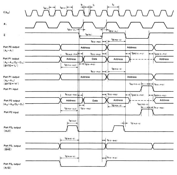
Memory expansion mode and microprocessor mode (When wait bit="1")
