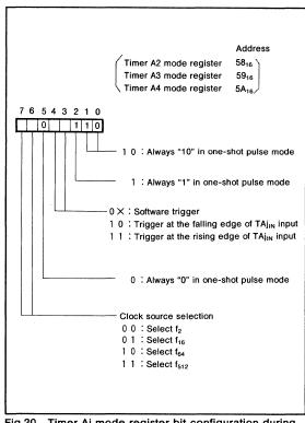
Fig.20 Timer Aj mode register bit configuration during one-shot pulse mode
