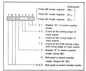
Fig. 29 Timer Bi mode register bit configuration during event counter mode
