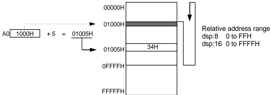
Figure 2.5.3 Address register relative addressing 1
