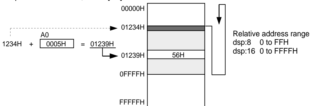
Figure 2.5.4 Address register relative addressing 2
