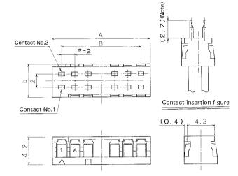
Note: The dip side may be deviated according to the cable thickness and the crimping contact bent up/down.
