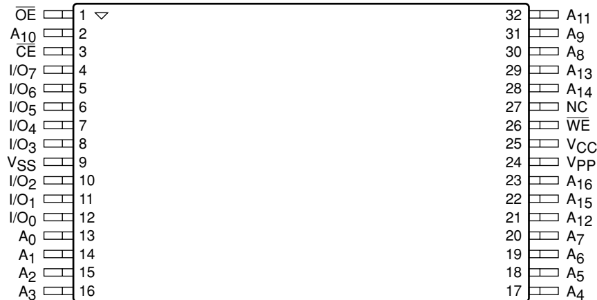
TSOP Package (Reverse Pinout) (TR, HR)
