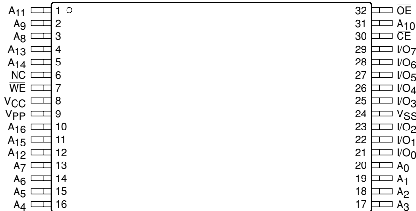
TSOP Package (Standard Pinout 8mm x 20mm) (T, H)
