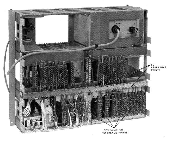
Fig. 2—Data Set 205C2, Rear View
