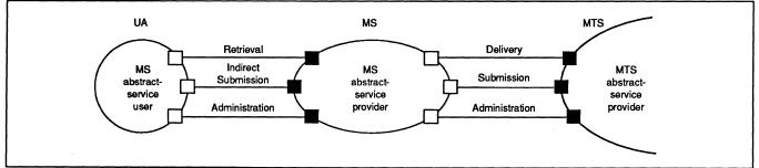
The MS object is an MTS user and, as such, the MS submission, delivery, and (MS-MTS) administration ports are consumers of the MTS-supplied service.
