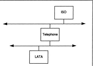
Under the OSI scheme, authorities assign ranges within a portion of the network address and can also assign lower portions of those addresses. This syntax is defined in the "OSI Addressing Syntax" section. The important concept is the hierarchy—the further down the hierarchy, the fewer bits have to be authorized (used). Currently, there seven authorities are recognized by ISO:
