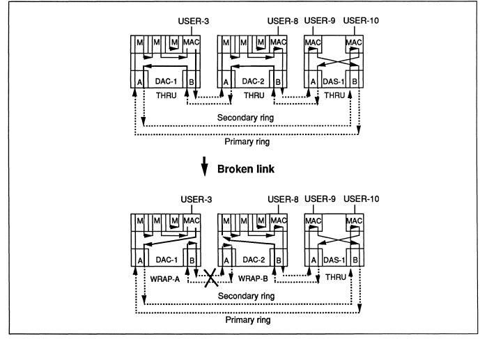
The net result is that all users end up on the Primary ring. The important point is that all users continue to communicate in spite of a break in the trunk ring.
