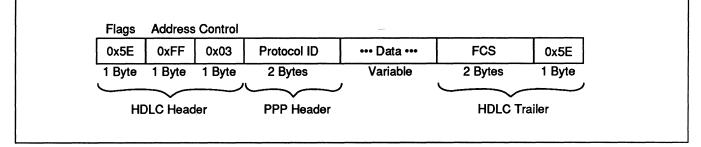
The flag sequence is the 8-bit value 01111110 (or 0x7E). The address and control fields defined in an HDLC frame will be set to 0xFF and 0x03, respectively. These settings mean that the HDLC address is not used and the frame type indicates an Unnumbered Information frame.
