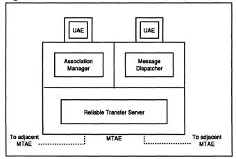
Here again, the layered concept is maintained; the RTS being responsible for the interaction with the session layer below it and providing a set of primitives for its interaction with the RTS user. The RTS is specified (X.410-1984) as an intercept on the development of what is now known as the Remote Operations Service Element (ROSE) and the Reliable Transfer Service Element (RTSE). The RTS is responsible for the complete and reliable transfer of MPDUs across a Session Layer connection.
