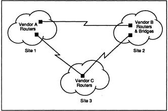
several sites that use equipement from different vendors are connected using point-to-point connections. PPP allows this environment to become an internet that is vendor-independent.
